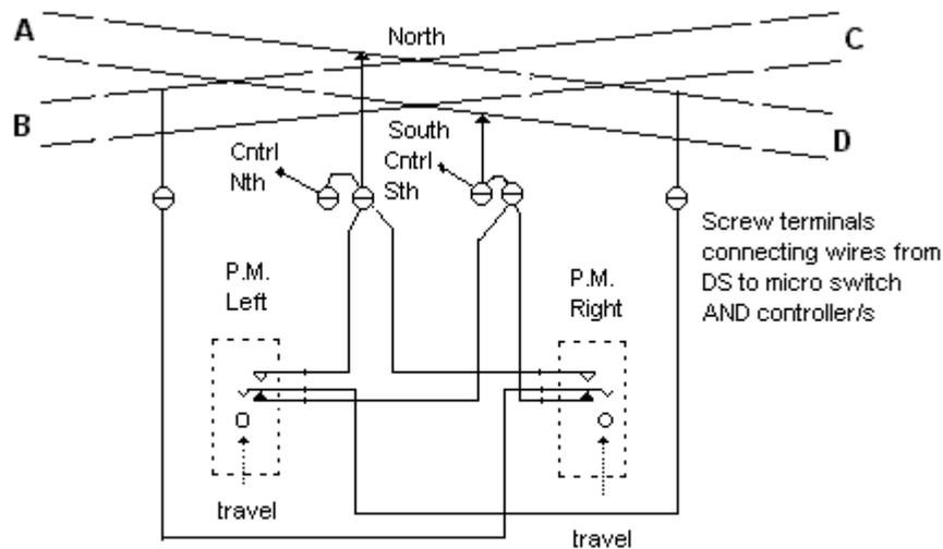
Double slip wiring diagram. Connections are correct for route setting A to C (Slip) and assumes that the armatures of both point motors are in the 'down' position. Note Controller must connect to the North and South terminals.
