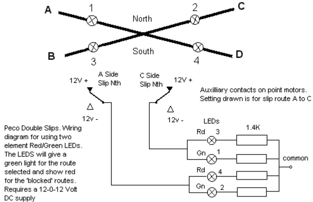
This circuit provides for four, Bi Color TWO ELEMENT LEDs to be mounted on your control panel to show which legs of the double slip are 'active' and which are 'blocked'.
