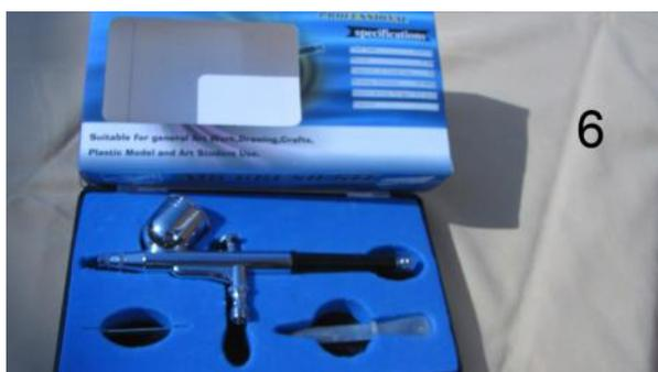
Only problem is that if you load it with a fair amount of paint for a bigger job and suffer a blockage, the cup takes several turns to release. Rather than do this and cover yourself in paint, disconnect the air hose and rotate the brush around the paint cup.
