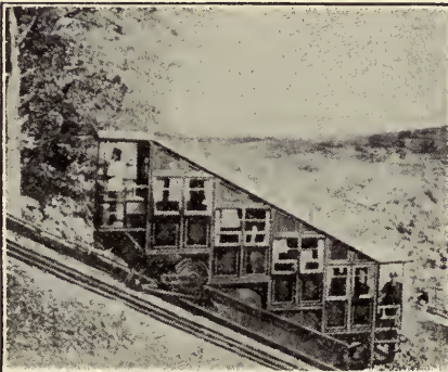
The Malberg railway at Ems is built to conform to the steep slope of the mountainside. The passenger compartment is built in a series of steps so that the seats are always upright.
