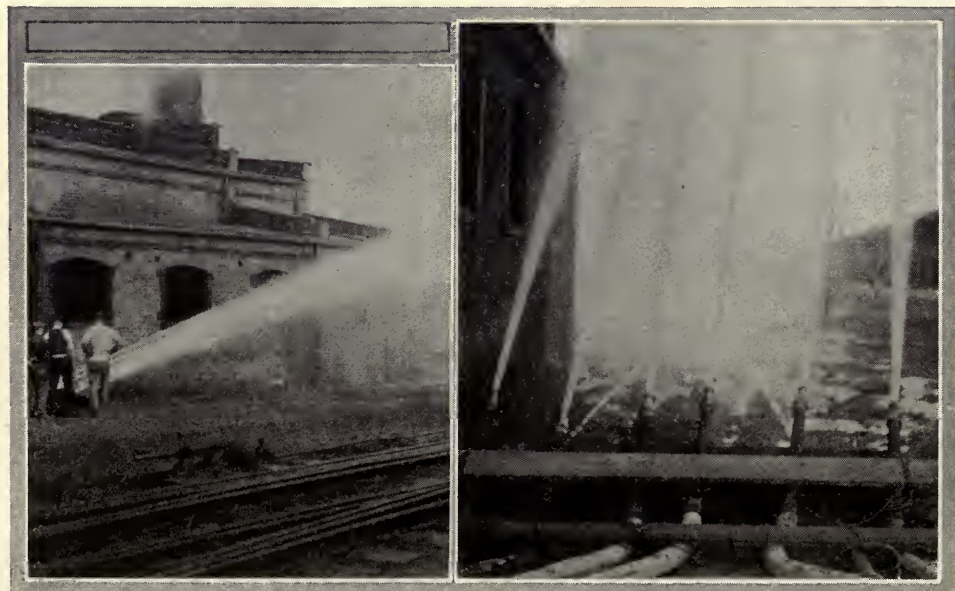
Fire protection test at our Stuyvesant docks, New Orleans, La. The six fire streams shown are throwing 1,800 gallons of water a minute.
