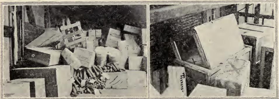
Causes of exceptions. At left, a car with no bulkhead after a heavy impact. At right, a heavy box loaded on top of a light one.
