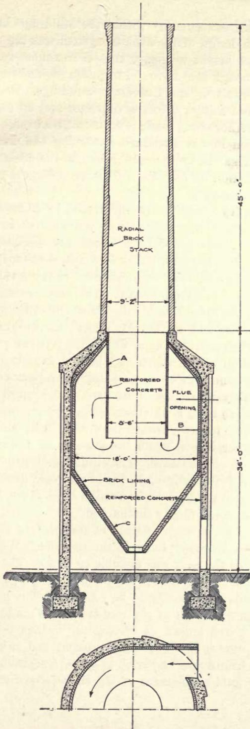
FIG. 55. CROSS SECTION THROUGH CINDER COLLECTOR AND STACK.
