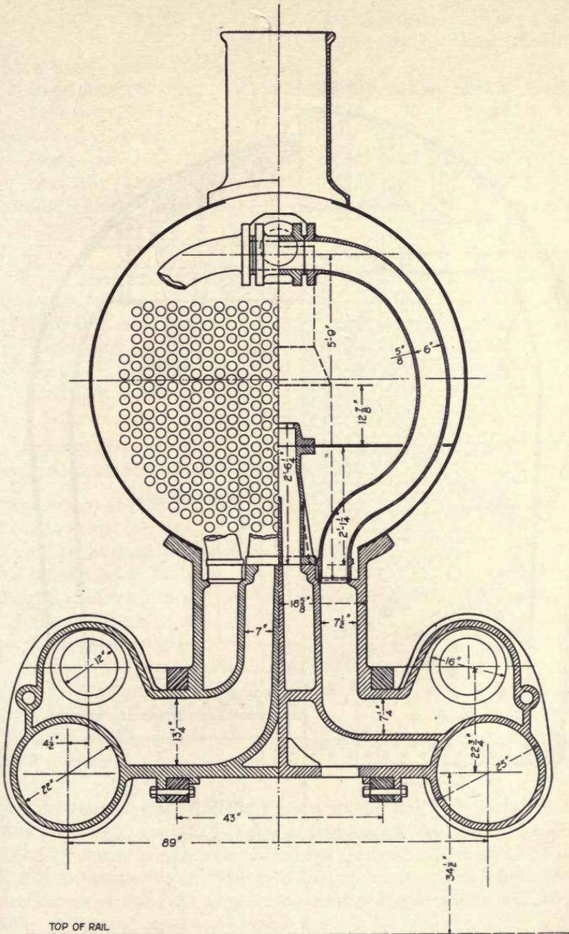
FIG. 43. CROSS SECTION THROUGH THE FRONT-END AND CYLINDERS.
