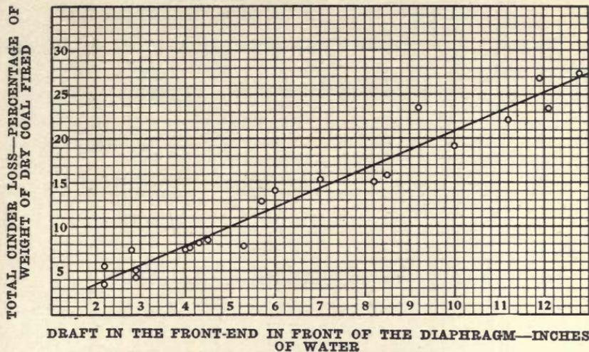
FIG. 14. THE RELATION BETWEEN CINDER DISCHARGE AND DRAFT.
