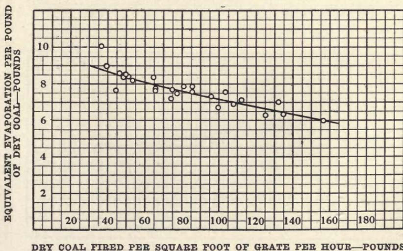
FIG. 32. THE RELATION BETWEEN EVAPORATION PER POUND OF COAL AND RATE OF COMBUSTION.
