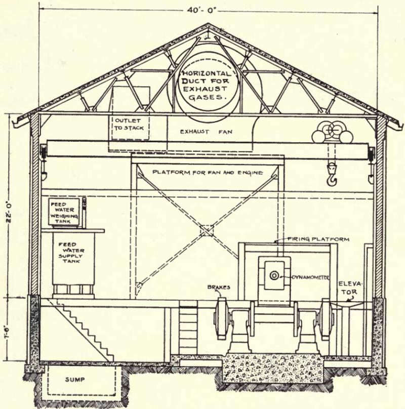
FIG. 54. A CROSS SECTION THROUGH THE MIDDLE OF THE LABORATORY.
