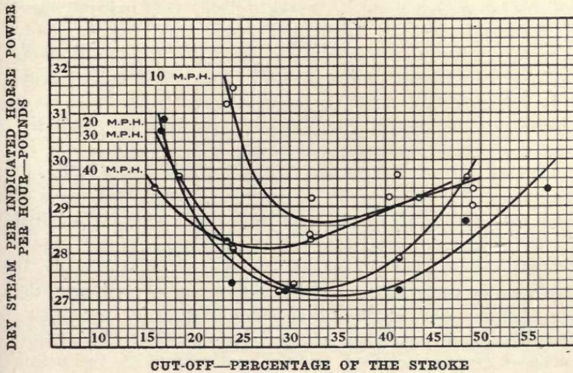
FIG. 18. THE RELATION BETWEEN STEAM CONSUMPTION AND CUT-OFF, AT VARIOUS SPEEDS.
