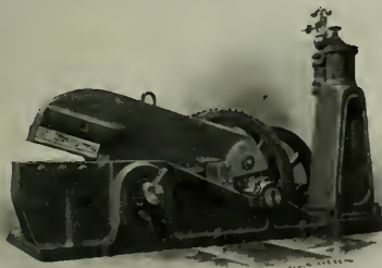
No. 5 SHEAR capacity 3 1-2" sq. cold Driven with 11 x 12 Engine.
