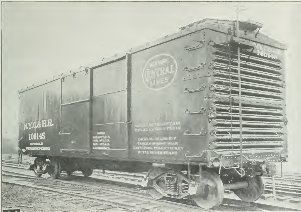
Steel End Applied to a New York Central & Hudson River Wooden Box Car.
