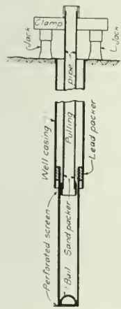
Method of "Sanding in" Well Casings.
