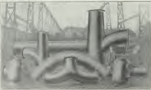
Examples of Large Heavy Piping Manufactured by Oxy-Acetylene Welding at the Works of A. Borsig in Tegel near Berlin.
