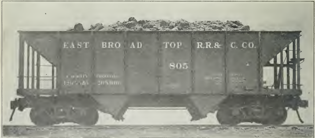
Narrow Gage All-Steel Hopper Car of 60,000 lbs. Capacity.
