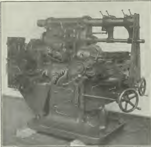
Universal Milling Machine, Motor Driven Through Spur Gearing.
