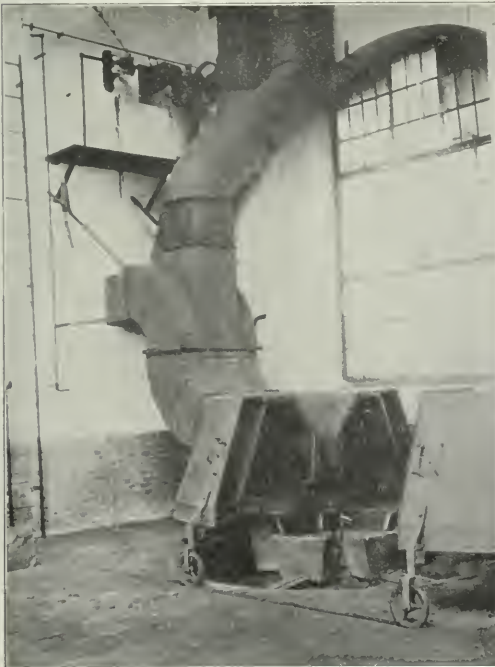
Locomotive Tire Heater in Roundhouse of Hungarian State Railways.
