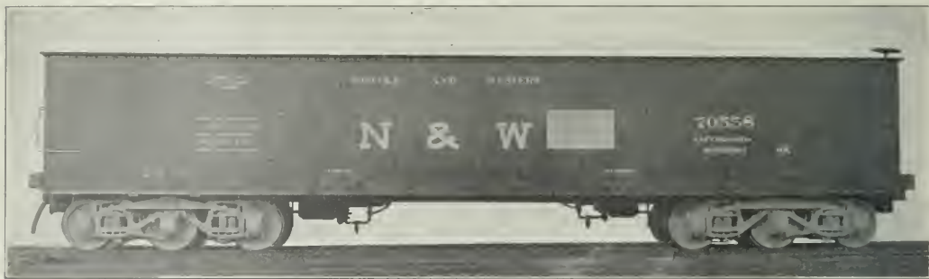
Ninety-Ton Gondola Car Mounted on a New Design of Six-Wheel Truck.
