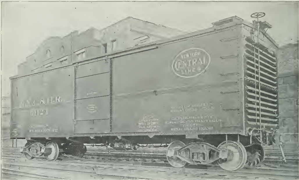
Experimental Steel Box Car on New York Central & Hudson River with Special End.
