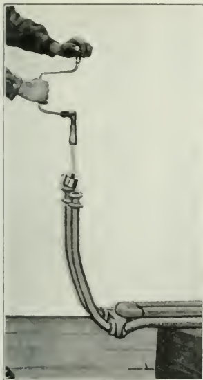
Tool for Finishing the Ball Ends of Superheater Units.
