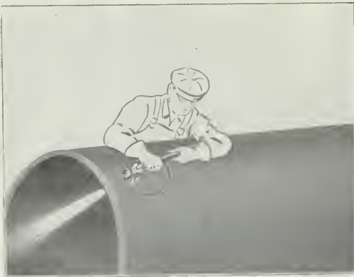
Cutting a Hole Through a Boiler Plate with an Oxy-Acetylene Torch.
