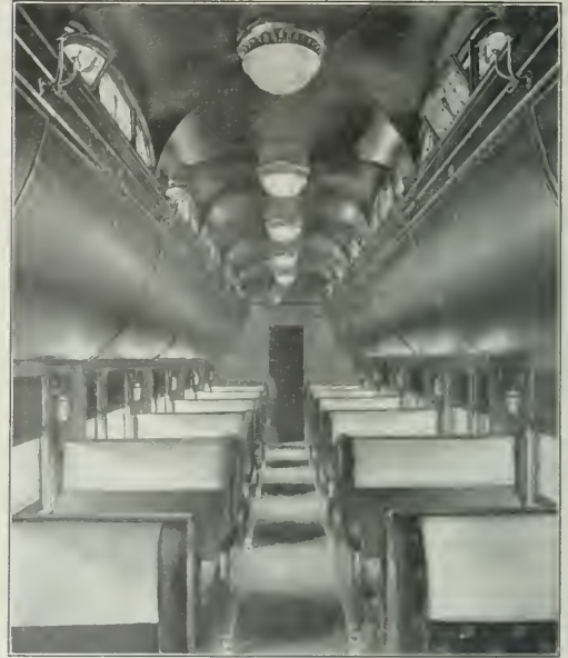
Canadian Pacific Sleeping Car Equipped with Pintsch Gas Light and Electrical Ignition.
