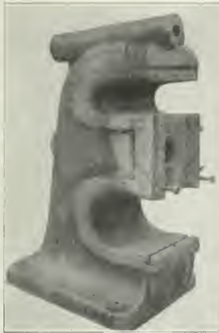
Main Base Casting of a Shear (Cast Iron) After Being Repaired with the Oxy-Acetylene Blow Pipe.
