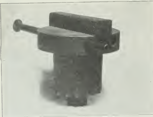
Revolving Portion of Alexander Crossing Frog, Showing Holes for Bolt Locking.
