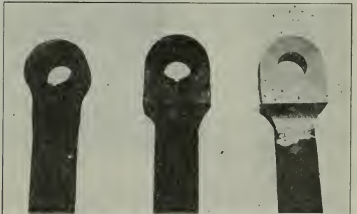
The Ends of Side Rods are Reinforced by the Oxy-Acetylene Process
