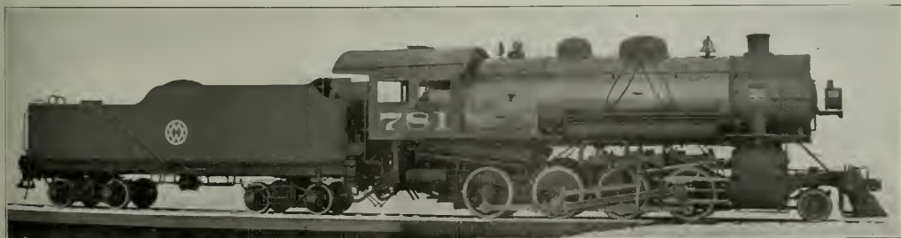
Western Maryland Consolidation Locomotive with 51 inch Drivers
