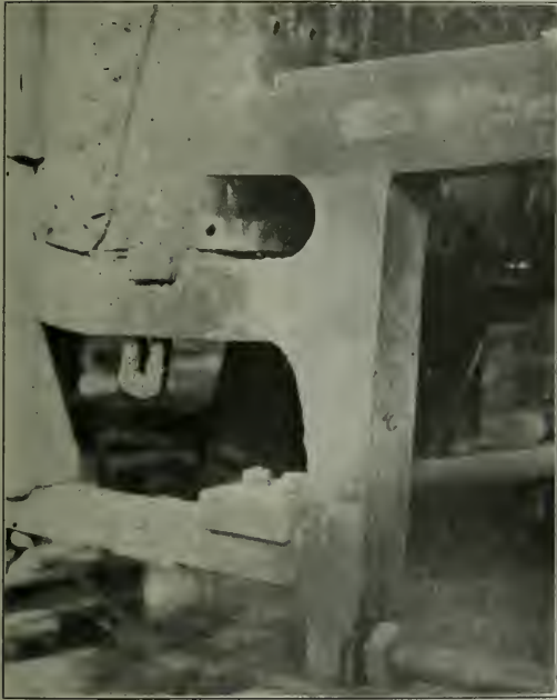
Pedestal Jaw Broken Between the Top and Bottom Rail Which Was Welded by Oxy-Acetylene Process
