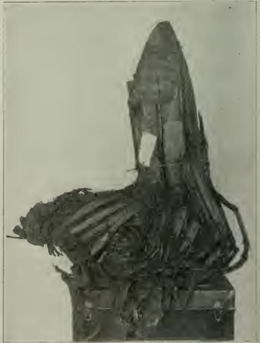
Creosoted Pile that Failed by Brooming About 3 ft. from the Point
