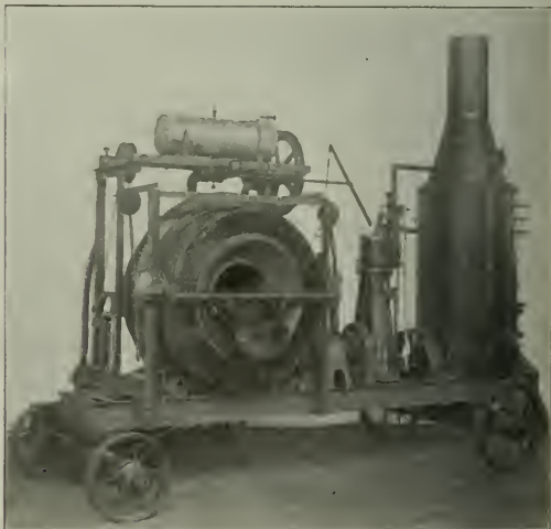
The Smith-Chicago Mixer with Steam Engine, Boiler, Power Charger and Enclosed Water Tank. The Chute is Shown in Discharging Position
