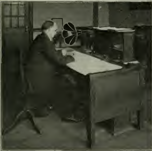
Despatcher's Desk Showing Loud Speaking Telephone Receiver
