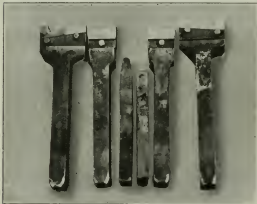
Tool Holder and Tools Now Used With Driving Wheel Lathe
