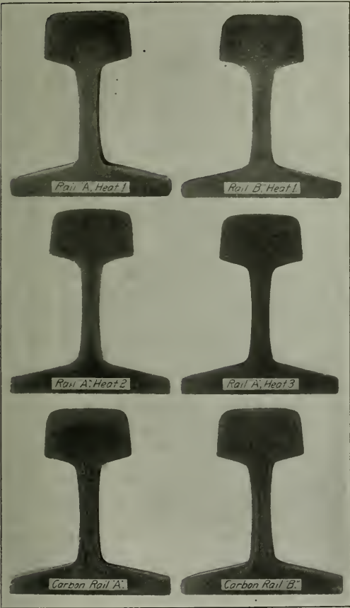
Etched Cross Sections of Vanadium and Carbon Steel Rails
