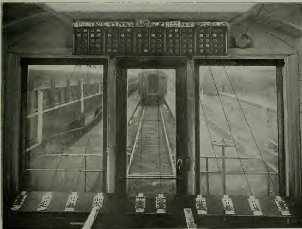
Observation End of Inspection Car Showing at the Bottom the Bank of Push Buttons Used by Observers in Registering the Grades and at the Top the Indicators Which Display These Markings. The Light Lines in the Cut Connect the Corresponding Push Buttons and Indicators
