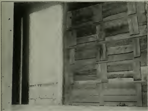
Fig. 7—Method of Closing Part of Side Door in Automobile Cars
