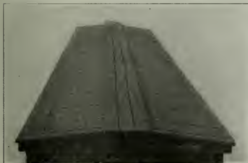
Fig. 2—Roof of Stock Car Equipped for Handling Grain
