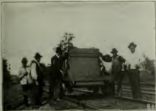
The Compressor Car with Machinery Enclosed Ready for Operation as an Ordinary Motor Car
