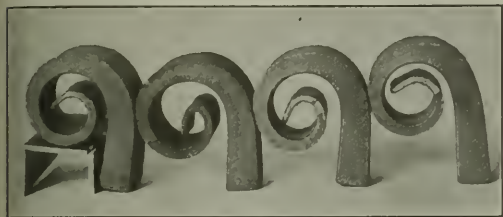
Malleable Iron Wedges Tested Under a Drop Hammer
