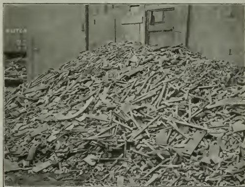
Fig. 2.—Wrought Iron Scrap Ready to Be Made Into Piles for Rolling Mill
