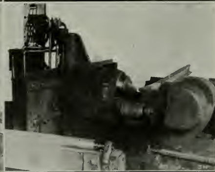
Above—Assembling and Riveting Together the Parts of a Frog
