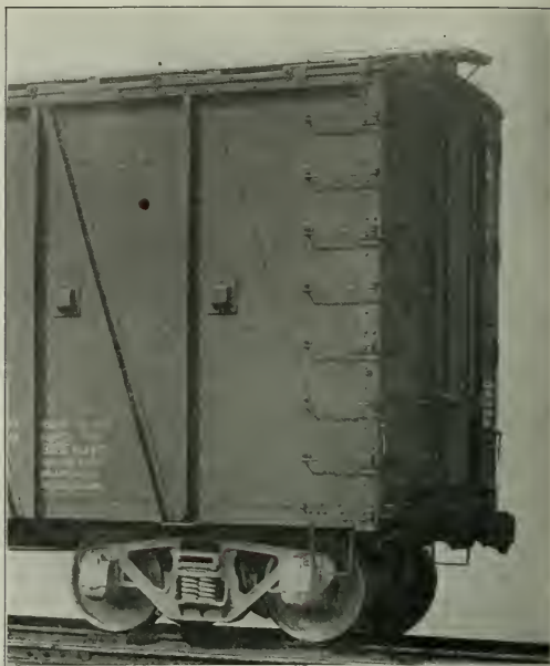
End of the Automobile Car Showing the Steel Doors
