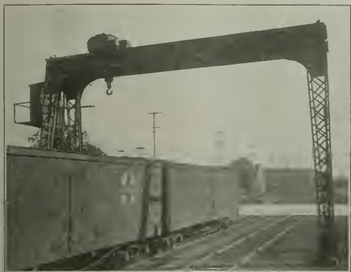
A 10-Ton Fixed Gantry Crane with Improved Type of Trolley and Hoist.
