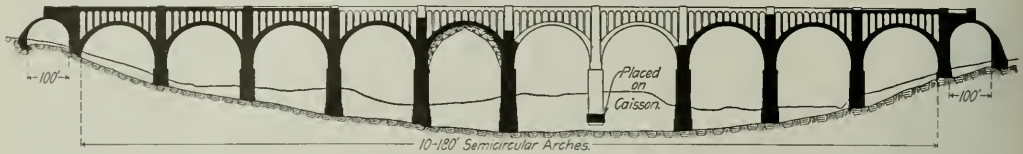
Outline Elevation of Tunkhannock Creek Viaduct Showing Progress up to January 1, 1915
