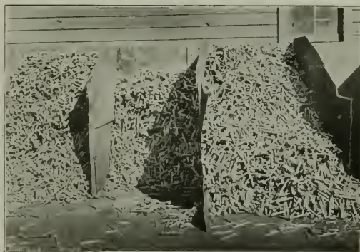
Fig. 8—Carriage Bolts Made on Automatic Bolt Machine
