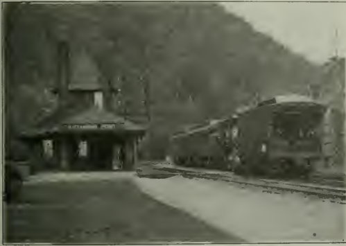
The Track Inspection Car on the P. R. R. Which Is Intentionally Made Hard Riding
