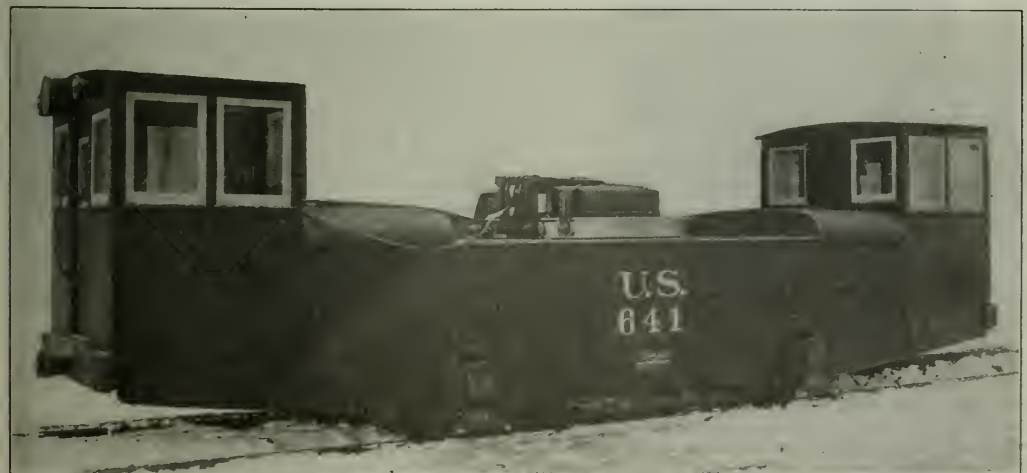
Electric Towing Locomotive Used at the Locks of the Panama Canal
