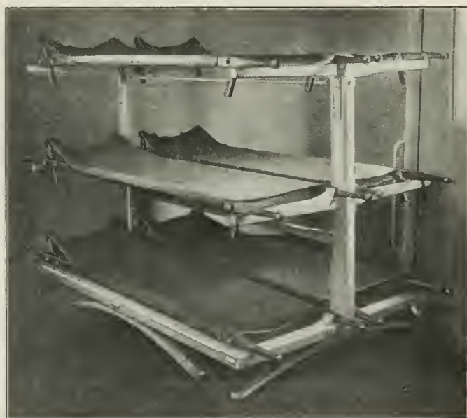
A Stretcher Frame Adapted for Use in Motor Ambulances or Freight Cars
