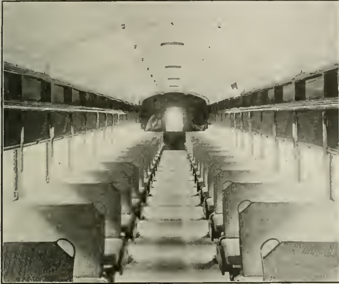
Interior of Long Island Steel Trailer Cars
