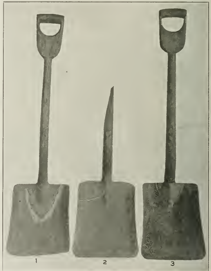
(1) Scrap Shovel with a Good Handle. (2) Scrap Shovel with a Good Blade. (3) A Serviceable Shovel Made by Piecing Together a Good Handle and a Good Blade Taken from Scrap Shovels
