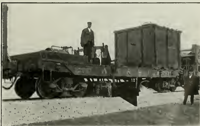
The Ballast Dresser and Sprinkler in Operation
