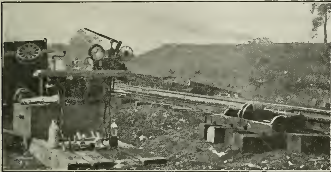
Track and Recording Apparatus for Measuring Lateral Thrust of Wheels on Rail
