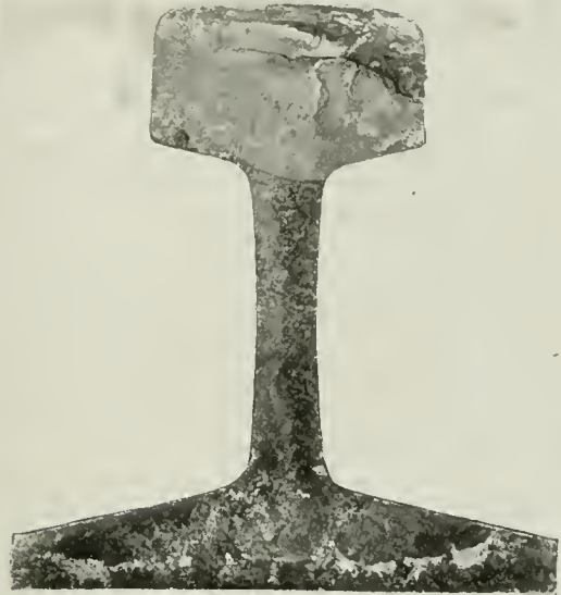
Fig. 21—Coalescent Type of Interior Transverse Fissure, Gagged upon the Head. The Crack or Nucleus Shows Beneath the Bearing Surface
