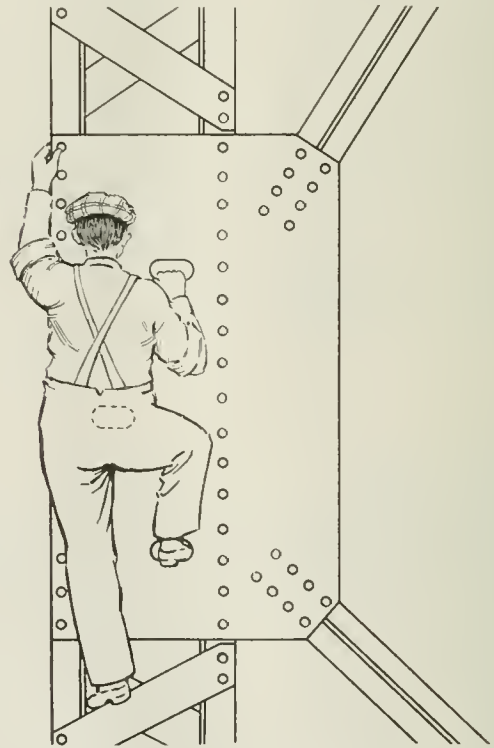
Sketch Showing the Use of Hand Holes in Gusset Plates
