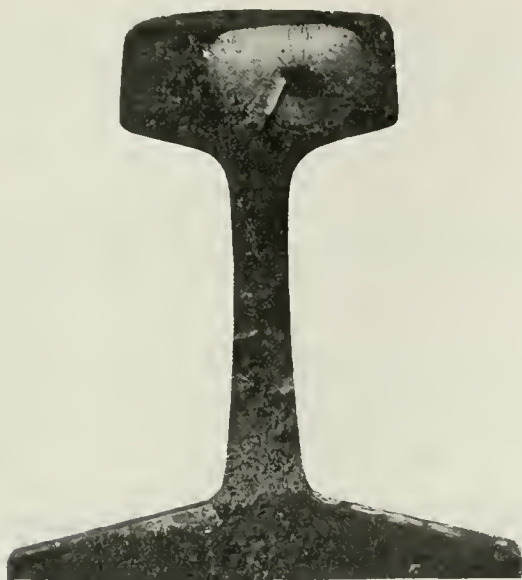
Fig. 18—Intergranular Type. This Illustrates the General Type of the Intergranular Nucleus and Is the More Common from the Fact That Rails Are Cambered as a Rule to Cool Low on the Hotbeds and Then Gagged Upon the Base
