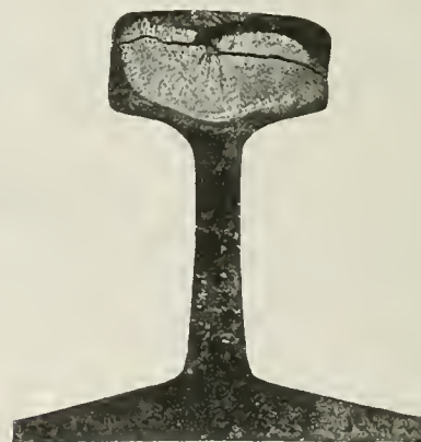
Fig. 19—Coalescent Type of Interior Transverse Fissure. Transverse View Showing the Nucleus—a Crack Under the Bearing Surface. Rail Gagged on the Head
