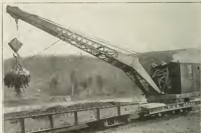
A 15-Ton Lehigh Valley Crane Mounted on an 8-Wheel Car Equipped with a Bent Boom and a 43-Inch Magnet
