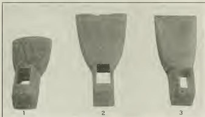
(1) Ground Down Until Worn Out. (2) Could be Put in Shape by Track Forces Without Being Sent to the Shop. (3) Has Been Reground Ready for Further Use
