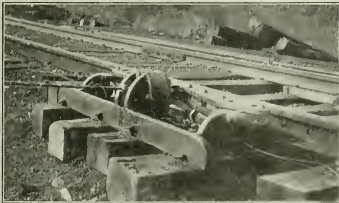
Lateral Thrust on Rails for Consolidation Locomotive Running at Different Speeds Over an 8 deg. 7 min. Curve Elevated for a Speed of 21.3 Miles Per Hour
