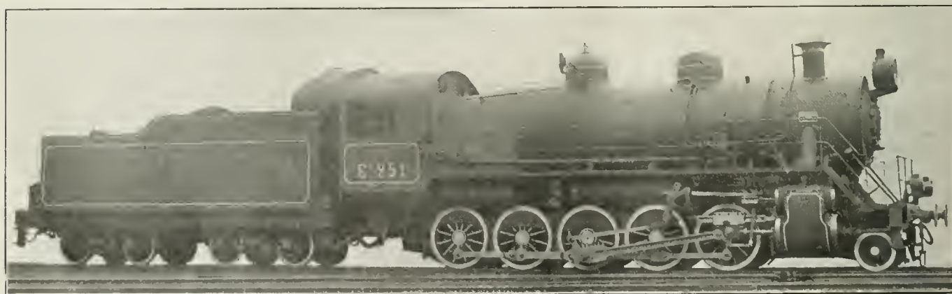
Decapod Type Locomotive Built by the American Locomotive Company for Russian State Railways
