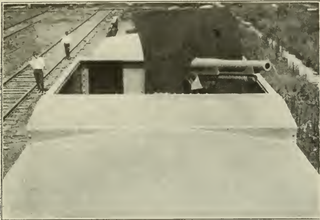
Top View, Showing the Gun-Well Equipped with a 3-in. Field Piece
