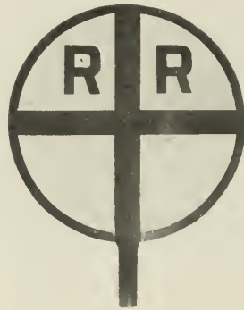
Proposed Distant Signal on Highways for Automobilists
