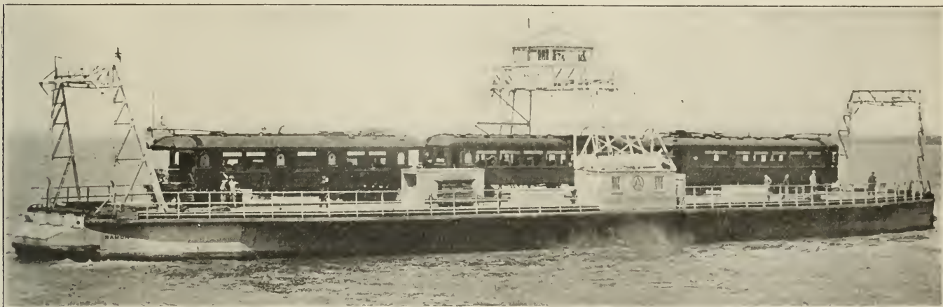
Car Ferry of the Oakland, Antioch & Eastern, Propelled by a Gasolene Engine
