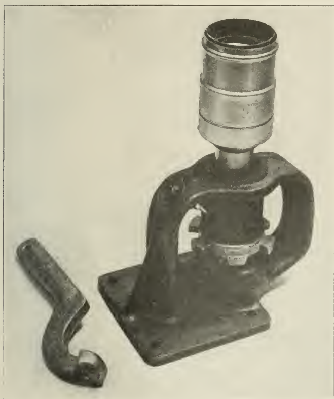
Fig. 5—Adjuster for Converting Oil and Arc Headlights to Incandescent
