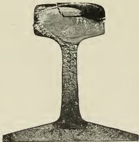
Fig. 4—Induced Interior Transverse Fissures. Coalescent Type. Rolled January 12, 1912; Failed January 16, 1915
