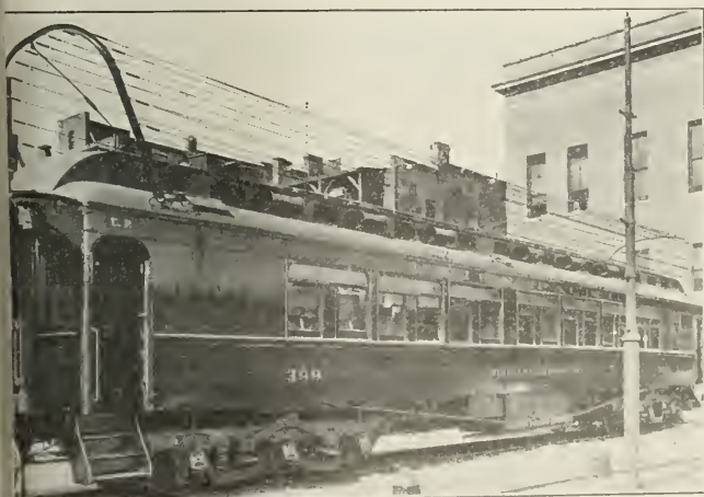
Car Fitted for Wireless Experiments on the Union Pacific
