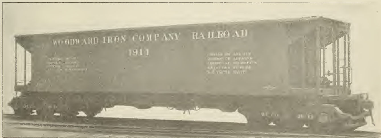
100-Ton Coal Car—Woodward Iron Company
