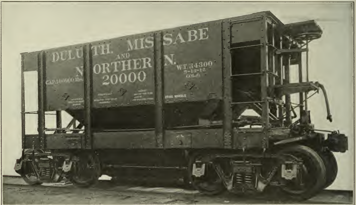
Steel Ore Car with Quick Operating Doors
