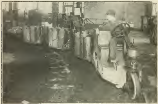
Fig. 4. One Man With an Electric Tractor Truck Can Haul Half a Dozen Loaded Trailers
