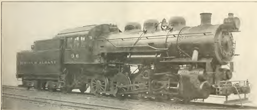
Boston & Albany Eight-Wheel Switcher Converted from a Consolidation Type Freight Locomotive
