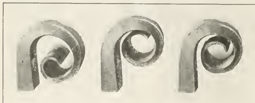
Fig. 3—Machined Malleable Iron Wedges Tested Under the Drop Hammer to Show the Ductility of the Core Metal
