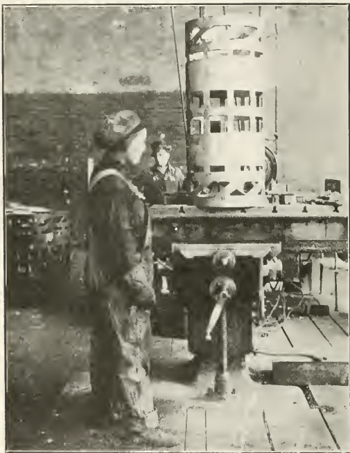
A Woman Operator Milling the Ports in a Valve Chamber Bushing, Pocatello Shops, Oregon Short Line
