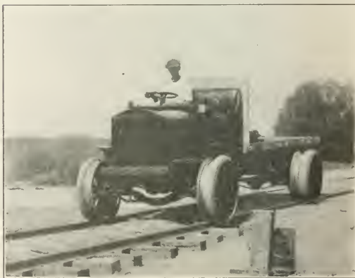
Auto-Rail Truck Mounted on the Rails
