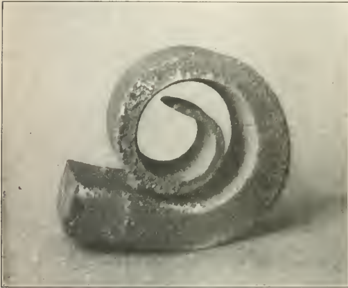
Fig. 1—Malleable Iron Wedge Tested Under a Light Drop Hammer
