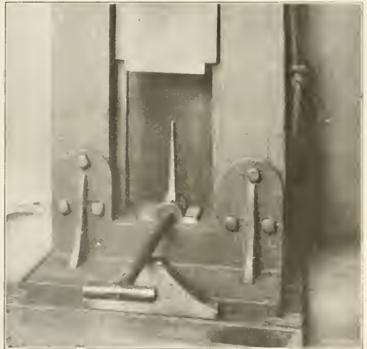
Fig. 2—Wedge Method of Testing the Ductility of Malleable Iron
