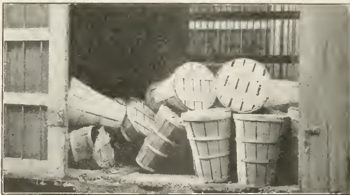
Not Enough Hampers Put Into the Car to Properly Brace Each Other
