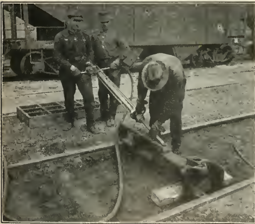
Removing Rivets from Drawbars with the Rivet Cutting Gun
