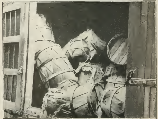
Damage Resulting from Only Partly Loading a Car
