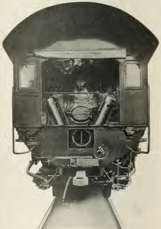
Cab View of a Locomotive Equipped with the Duplex Stoker
