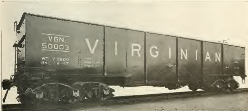
Virginian 120-Ton Flat Bottom Coal Car Built by the Virginia Bridge & Iron Company
