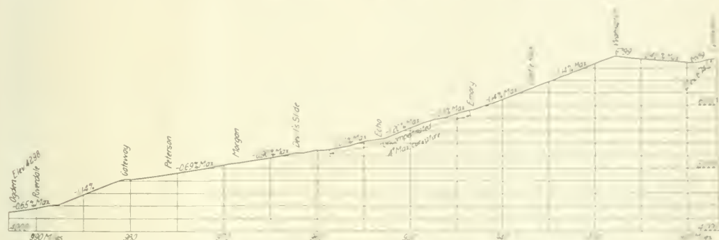
Profile of the Union Pacific Between Ogden, Utah, and Evanston, Wyoming
