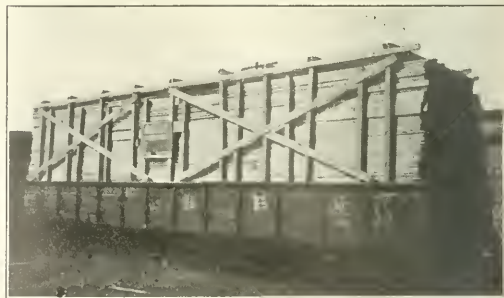
Car of Lumber Loaded to 110 Per Cent of Marked Capacity
