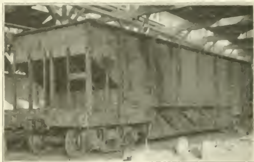
Sides and Ends in Place Ready for Application of Doors and Appliances
