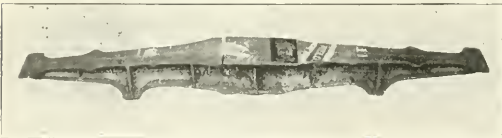
Fig. 6—Book B, Test 16. Body Bolster Welded in Tension Member, Broken in Tension Member Outside the Weld
