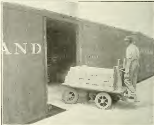
Electric Trucks Can Operate In and Out of Box Cars
