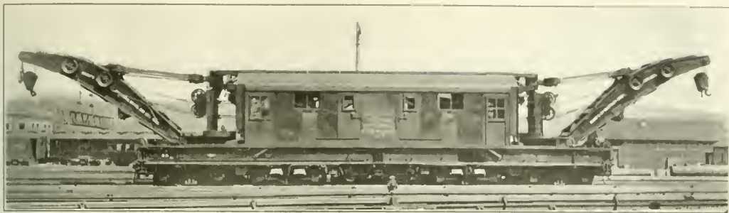
Double-End Electric Crane Independent of Road Rail or Trolley
