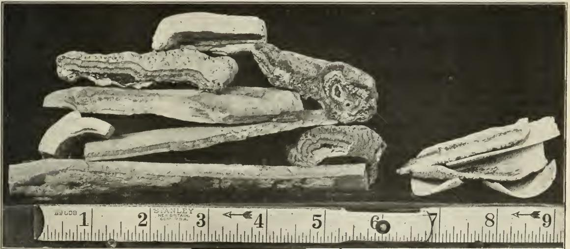
Samples of Scale Produced by Water That Had Seeped Through the Cinder Fill
