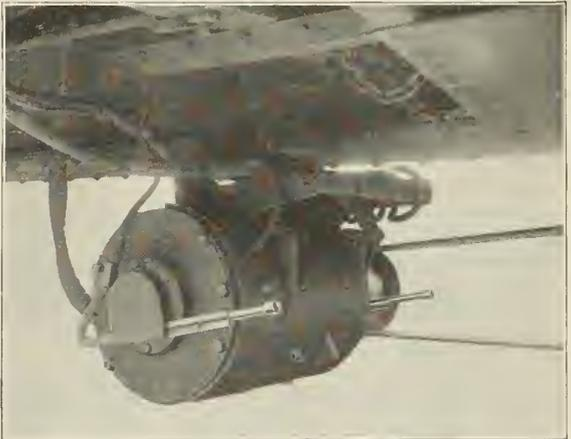
Generator with Thermometers Applied to Bearings
