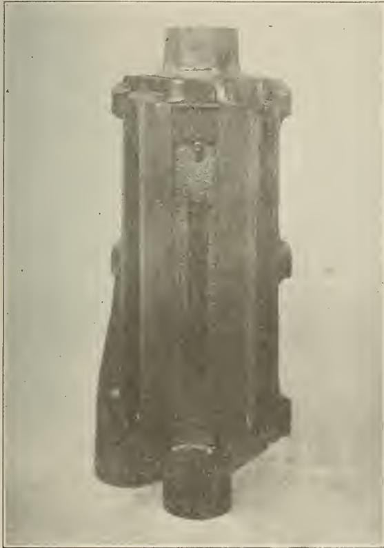
Babcock Water Gage Protector with a Slot in the Casing to Illuminate the Interior
