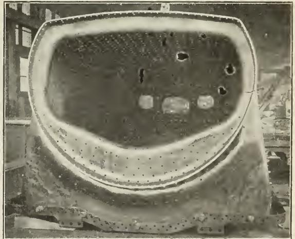
The Firebox and Combustion Chamber Connection Sheet
