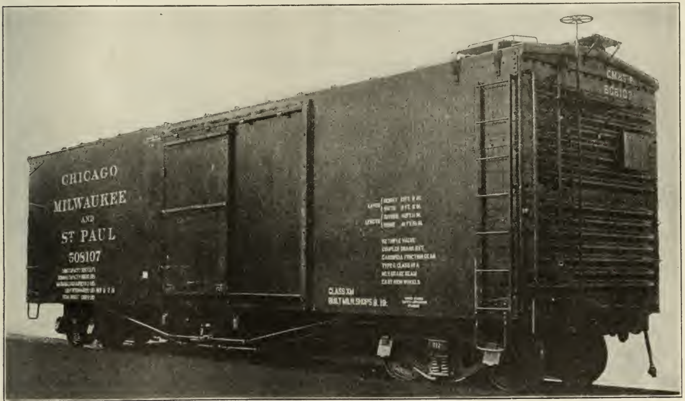
Double Sheathed 40-Ton Capacity Box Car Designed and Built by the C. M. & St. P.
