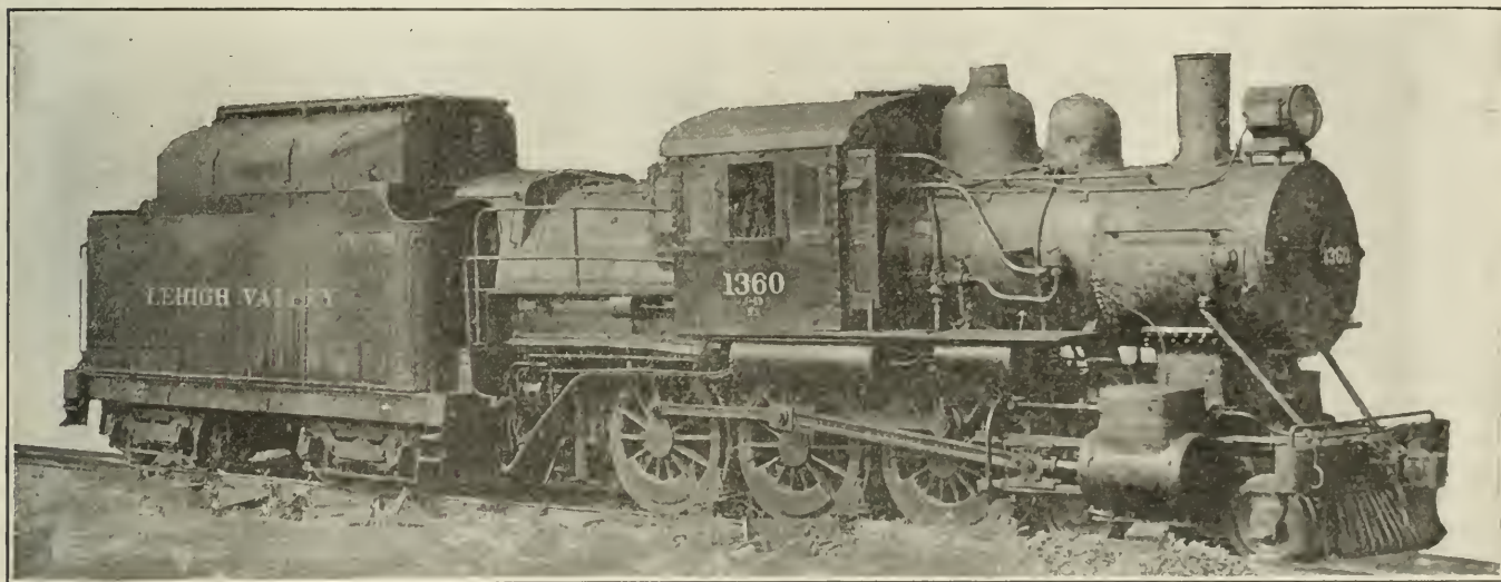
Lehigh Valley Locomotive Equipped with Pulverized Fuel Burning Apparatus
