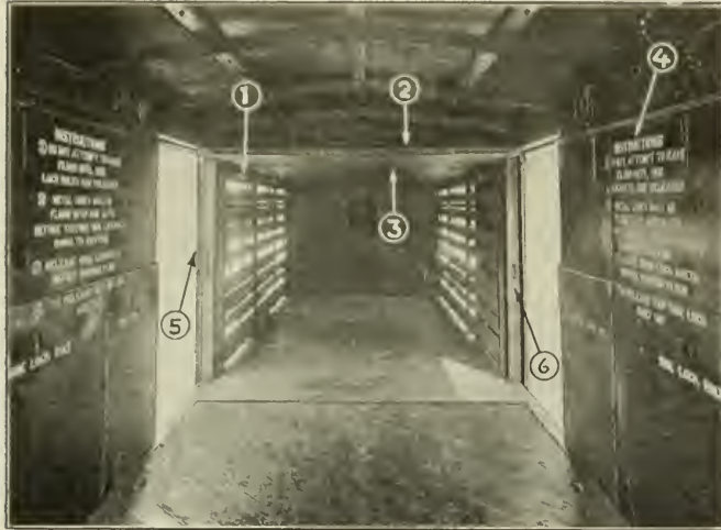
Fig. 2—One End of Car Arranged for Merchandise. (1) Safety lock; (2) Moveable floor; (3) Showing absence of any nails or projections to injure live stock; (4) Instructions for operating device; (5) Door water seal; (6) Provision for fastening grain doors.
