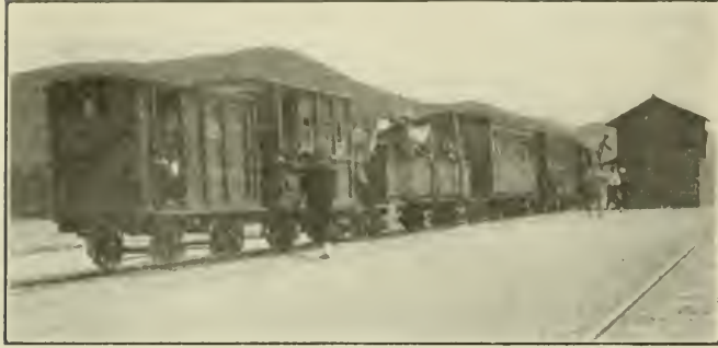
Typical Light Railway Equipment Such as Is Used on the 2 Ft. 6 In. Gage Feeder Lines of Japan, Korea or Formosa
