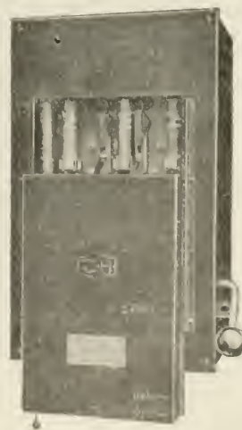
Lowering the Panel of the Three-pole Starting Switch Deadens the Fuses and Makes Them Accessible for Renewal
