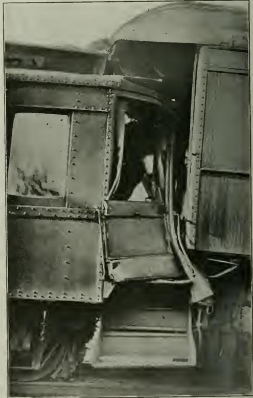
First Stage of Telescoping of Steel Cars
