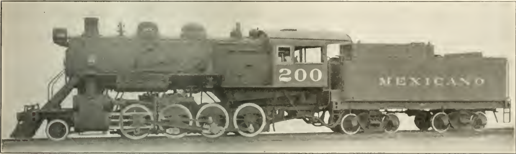
Standard Gage Consolidation Locomotive for Mexican Railway
