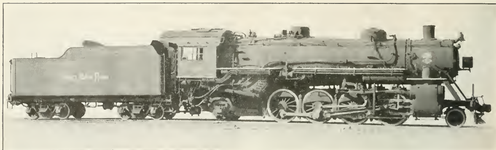
Mikado Locomotive Equipped with Booster
