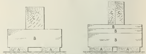
Lumber Bearing Built of Sound Salvaged Material
