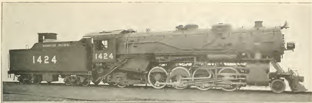
Mikado Type Locomotive Equipped with Booster
