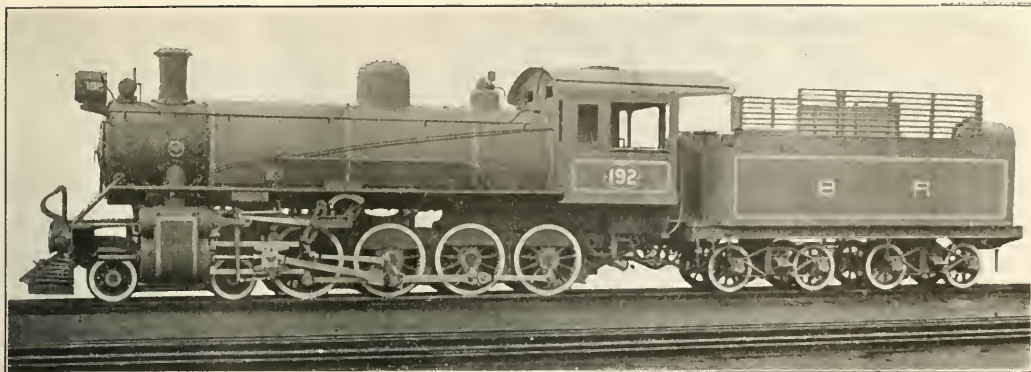
Benguella Locomotives Are Equipped with Automatic Vacuum Brakes
