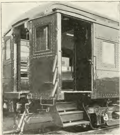
Air-Operated Sliding Doors Are a Feature of the Vestibule Design
