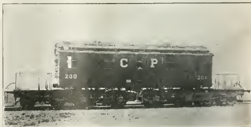
120-Ton 3,000-Volt Passenger Locomotive
