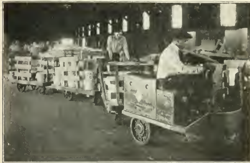
When Long Hauls Are Necessary, the Trailing Method of Handling Is Used
