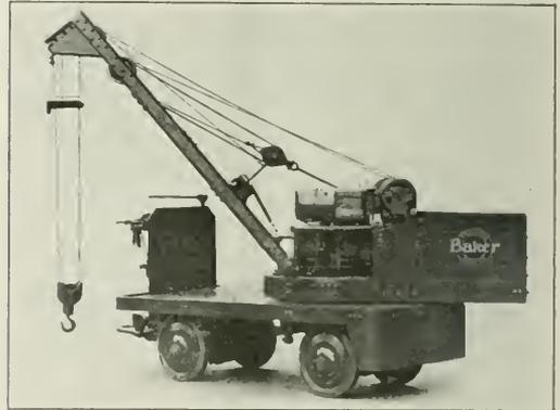
Three-Movement Electric Crane Truck
