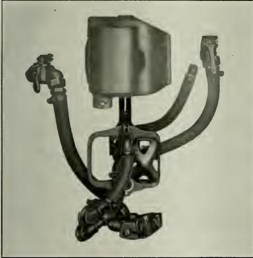
Face of Passenger Connector Head; Brake Pipe and Signal Adapter Is Attached Direct to the Head, Steam Heat Adapter to the Hose
