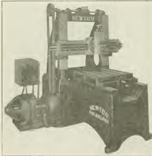
View Showing Motor Drive Arrangement
