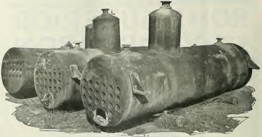
*These boilers, removed because of a recently enacted state law prohibiting the use of boilers after 30 years' service, were fitted with boiler tubes made of Parkesburg Charcoal Iron. After 40 years of service, these tubes of Parkesburg Charcoal Iron are in almost perfect condition.*
