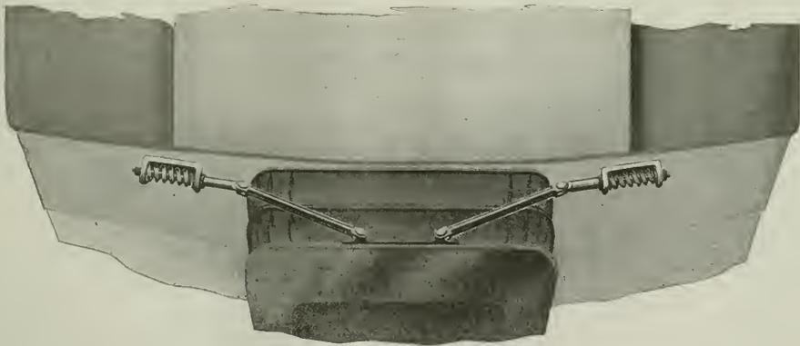
Outside Connected Top Diaphragm Buffing Mechanism
