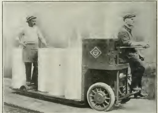
The Truck Is a Drop-Frame Truck of Special Design
