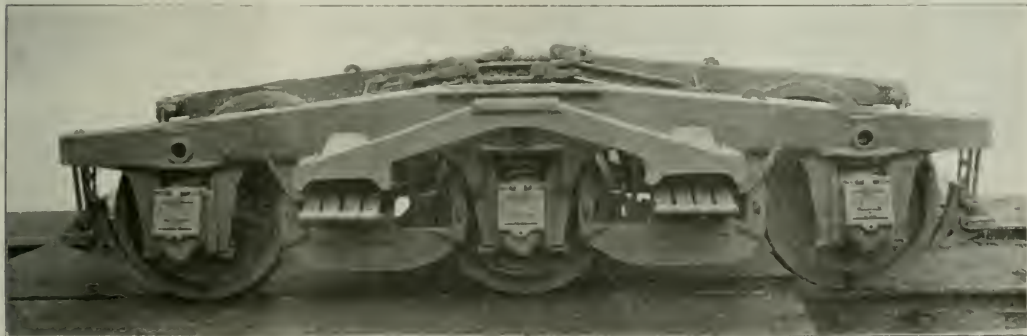
Cast Steel Side Frames Reduce the Weight of the Truck and Decrease the Number of Parts
