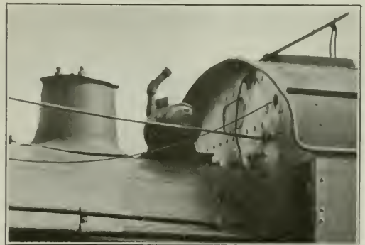
Typical Installation of Headlight Unit on the Buffalo, Rochester & Pittsburgh Railroad Locomotive
