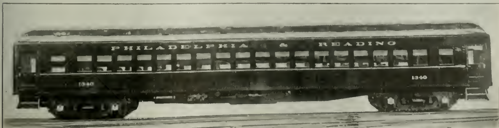
New 63-ft. Steel Coaches for the Philadelphia & Reading
