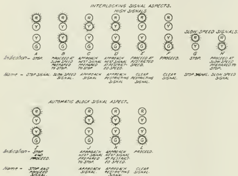
Interlocking and Automatic Block Signal Aspects
