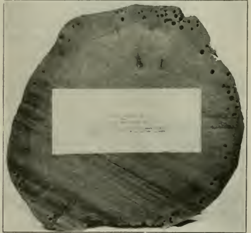
Section of an Untreated Pile from Lehigh Valley Pier at Jersey City after Ten Year's Service Indicating Recent Attack. Living Organisms Were Extracted from This Pile in September, 1922
