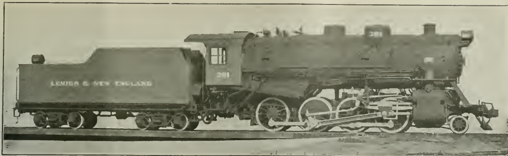
Consolidation Locomotive Weighing 301,500 lb. and Having a Tractive Force of 68,200 lb.
