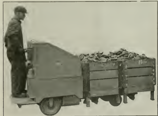
The Elevating Platform Adds Greatly to the Labor Saving Possibilities of the Truck
