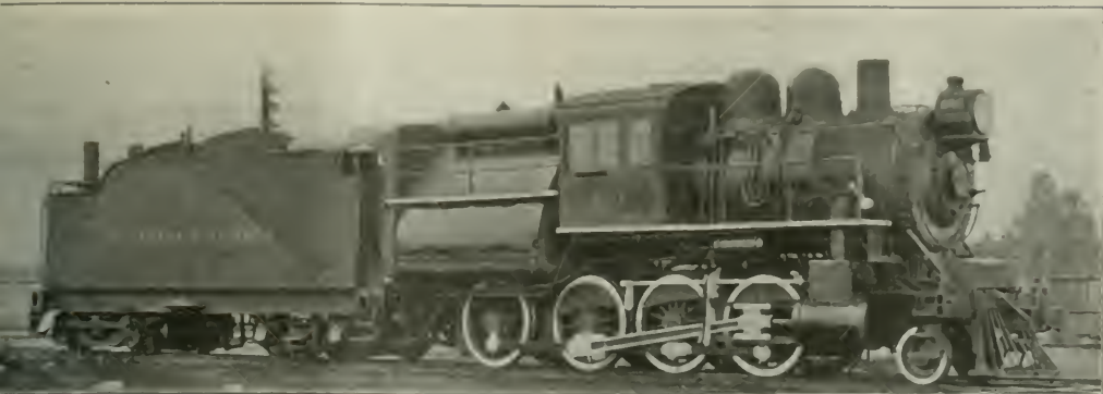
Superheated Consolidation Locomotive to Which the Tender Booster Has Been Applied
