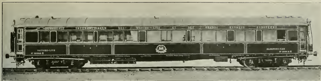
All-Steel European Sleeping Car Built by Leeds Forge Company, Ltd.
