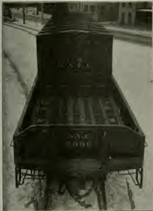
Container Cars for Mail Service Have a Wire-Mesh Floor
