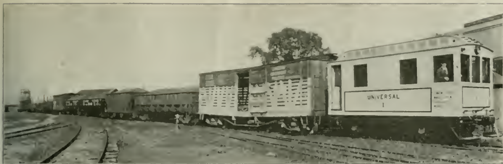
Hauling 14 Cars Weighing 645 Tons with a 150-Horse Power Gasoline Locomotive.
