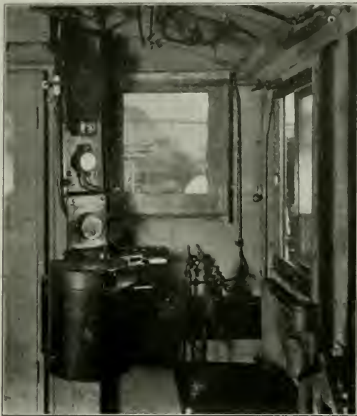
Interior of Operating Cab, Buenos Aires & Western Locomotive, Showing Master Controller, Brake Valve and Instrument Panel
