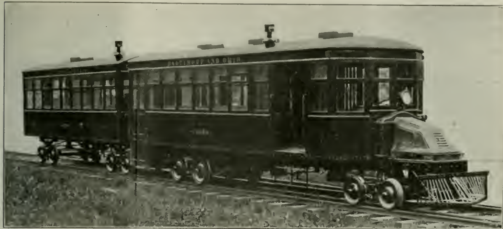
Edwards Motor Car Unit with Seating Capacity for 56 Passengers
