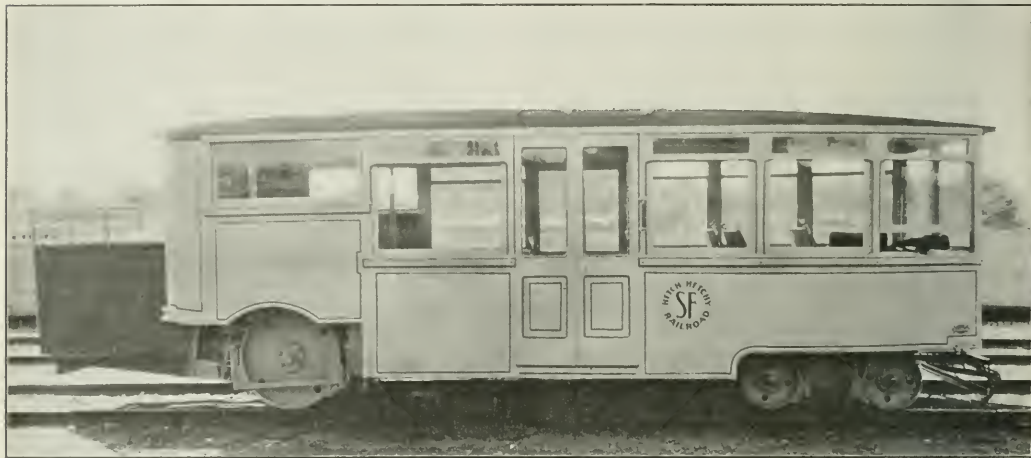
The Location of the Engine at the Rear of the Body Is a Distinctive Feature of This Car
