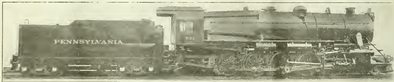
DECAPOD OR 2-10-0 ON THE PENNSYLVANIA RAILROAD.
