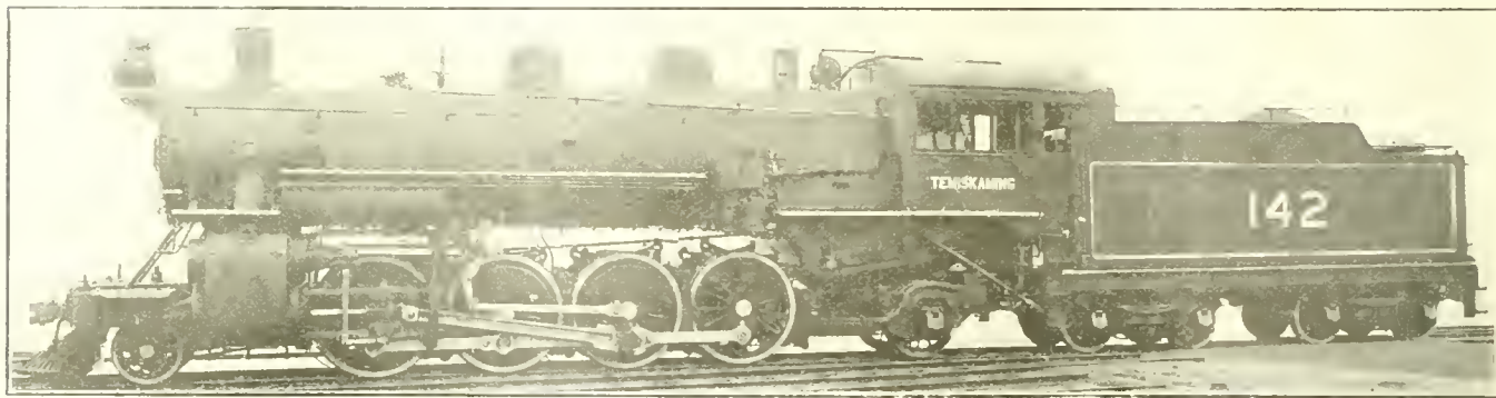
2-8-2 FOR THE TEMISKAMING & NORTHERN ONTARIO RAILWAY.
