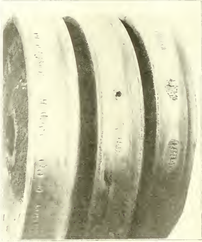
FIG. 1. EXCESSIVE BRAKE BURNING AND COMBY TREAD.
