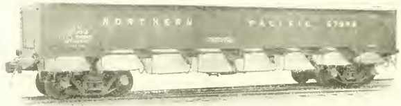
FIG. 2. GONDOLA WITH DUMP DOORS OPEN.
