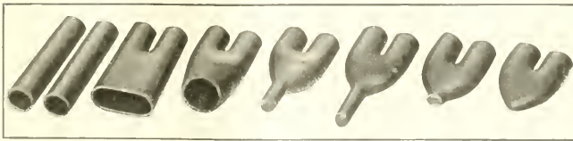
FIG. 1—FORGED RETURN BEND, SHOWING THE STEPS IN THE MANUFACTURING PROCESS.
