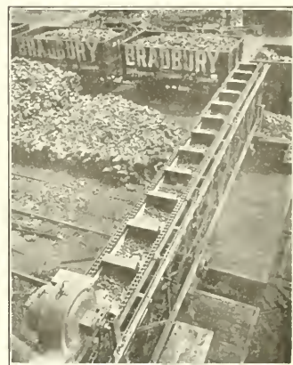
CONVEYOR HANDLING COAL.
