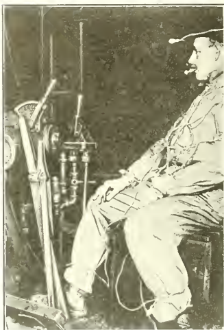
ENGINEMAN AS HE SITS IN CAB WITH TARGET REVERSE LEVER.
