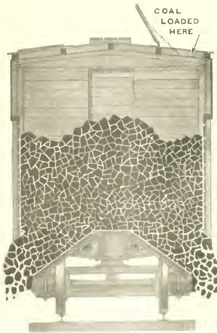
BOX CAR WITH HOPPER DOORS IN FLOOR, CARRYING ROUGH FREIGHT.
