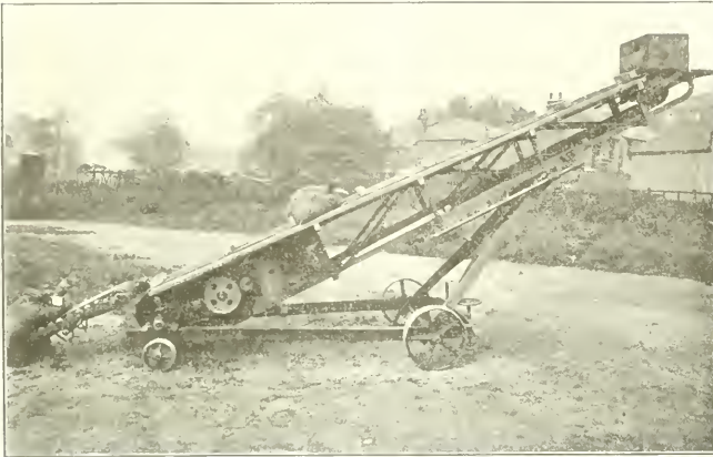
THE "BOOSTER," MOTOR USED WITH GRAVITY CONVEYORS.
