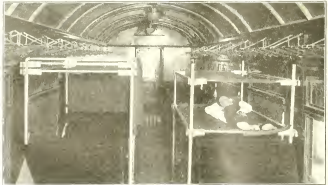
COVINGTON'S DEVICE FOR TRANSFORMING A DAY COACH INTO A SLEEPER FOR MILITARY TRANSPORT SERVICE.
