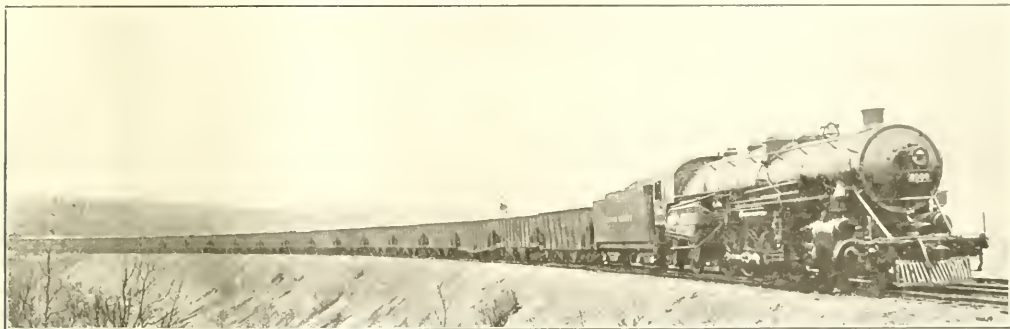
LEHIGH VALLEY RAILROAD COAL TRAIN DRAWN BY LOCOMOTIVE USING MIXED PULVERIZED FUEL
