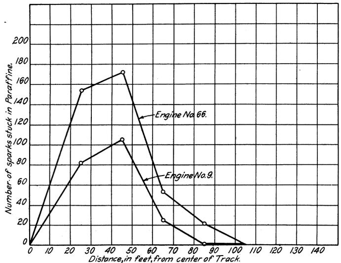
Fig. 3.—Total number of sparks that stuck in the paraffine for both locomotives
