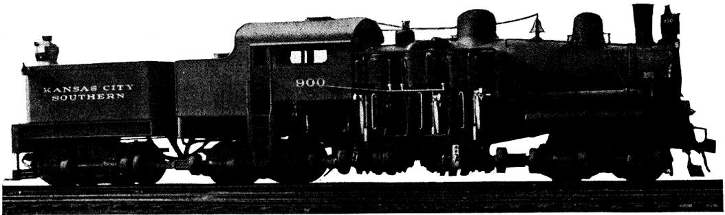
FIG. 1. 190-TON GEARED LOCOMOTIVE FOR SWITCHING SERVICE ON 7% GRADES AND 60° CURVES; KANSAS CITY SOUTHERN RY.
