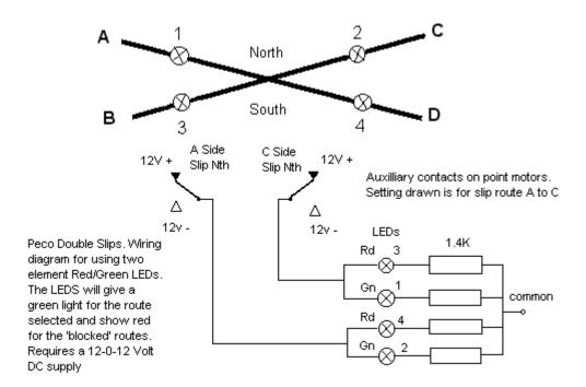
This circuit provides for four, Bi Color TWO ELEMENT LEDs to be mounted on your control panel to show which legs of the double slip are 'active' and which are 'blocked'.
