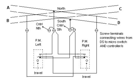
Double slip wiring diagram. Connections are correct for route setting A to C (Slip) and assumes that the armatures of both point motors are in the 'down' position. Note Controller must connect to the North and South terminals.
