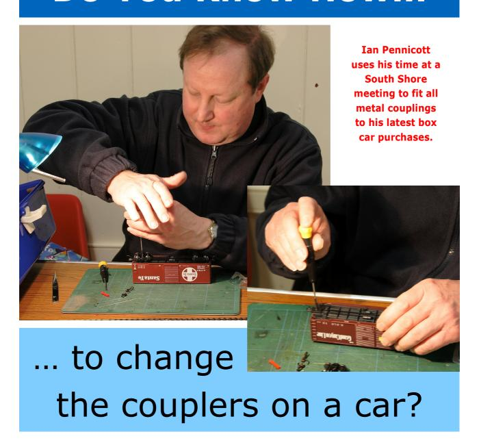
Smooth switching operation relies upon easy coupling and uncoupling. Ensuring a constant standard makes this task simpler. Just one of the 'simple' pieces of NMRA member shared know-how
