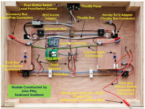
John Pitty made this demonstration board to show how an electrical diagram is converted into the real life product used for controlling a module.
