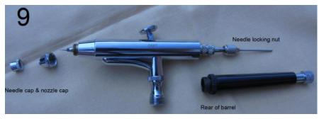
no need to undo the other knurled nut - it holds in a big spring and the trigger. Took ages to figure out how
