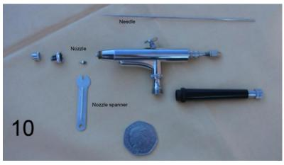
to reassemble that lot. So undo the needle cap and nozzle cap from the front. In fact they frequently come off as one. Clean, especially rind of paint in nozzle cover.
