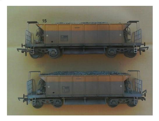
Factory weathered Mk1 coaches. (Photo 16.) As with the seacows these had a very basic weathering applied along the sides, but not the ends. The colour underneath has been varied and weathering applied to the ends.
