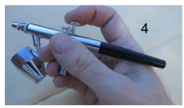
One simply identified as BD-128. (Photo 4.) Seems ok, but trigger operation doesn't seem as smooth as it might be. The paint cup fits under the barrel at a strange angle. I assume it is intended for spray tanning. The position of the cup makes it difficult to hold the airbrush comfortably and it takes a comparatively large amount of paint to cover the tube coming out of the paint cup. As with the others it's dual action (press for air, pull back for paint),
