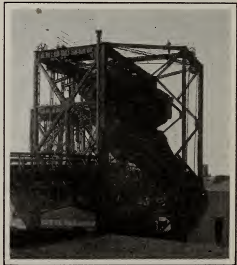
THE CAR DUMPER TURNS A GONDOLA UPSIDE DOWN
