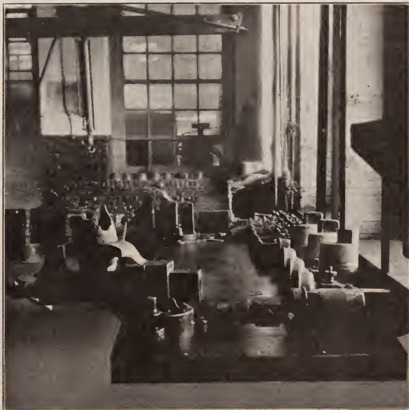
Properly located and arranged branch in Automatic Department, Mt. Clare, which is used for assembly of such parts as relief valves, toggle joints, whistles, etc.
