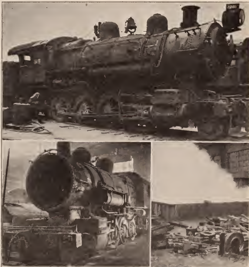
Above: Engine being sand blasted on dead line, Glenwood. Below, left: engine on stripping pit, Glenwood. Right: Lye Vat, Glenwood, in which all material taken from locomotive, requiring repairs and testing, is cleaned
