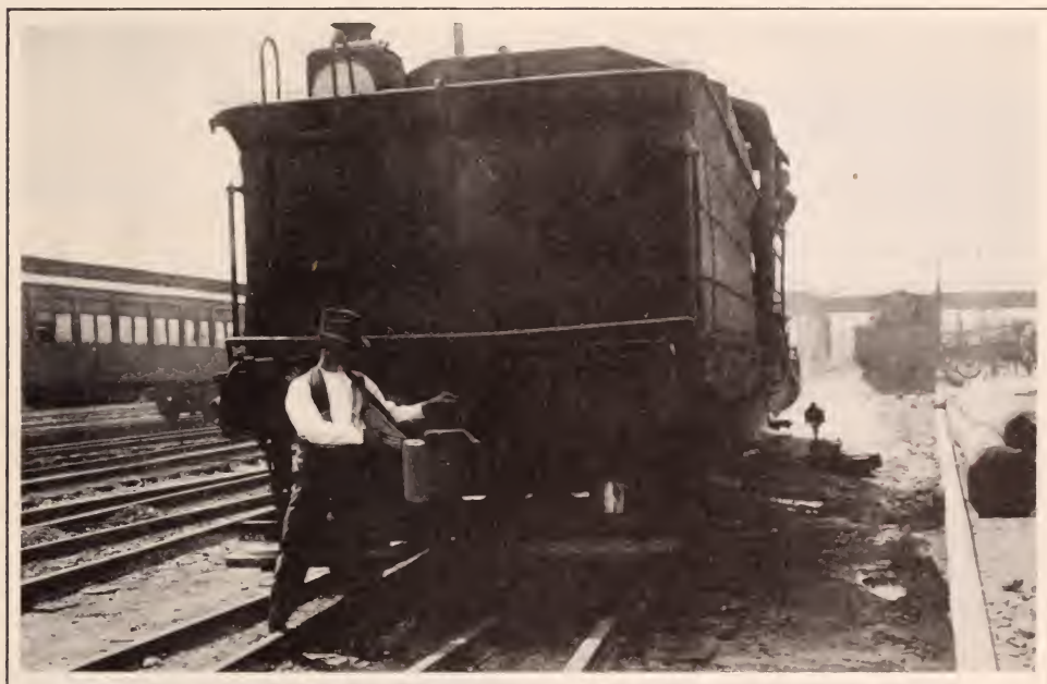
VEST CAUGHT IN OPENING KNUCKLE—AN AVOIDABLE CAUSE OF ACCIDENT
