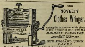
It has Cog Wheels on both ends of the Rolls, which allows the rolls to separate at either end. The Patent CURVED CLAMP has a bearing on a tub the whole length of the Wringer. With our Patent Adjustable Springs, only one pressure screw is required, which always insures an equal pressure the whole length of the rolls, and makes the Wringer Self-adjusting and adjustable. Altogether it is the most Durable, simple and efficient Wringer in use. Warranted perfectly satisfactory. Sold everywhere.
