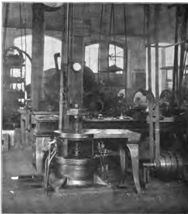
Device for Inserting and Removing Driving Box Brasses.
