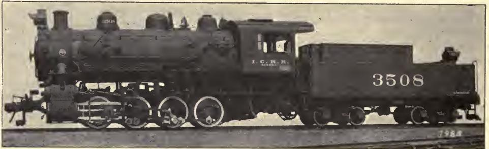
Herewith is reproduced a photograph of one of the new switch engines. Twenty-five of these engines are being purchased by the Illinois Central from the Baldwin Locomotive Works. They are the largest switch engines in use on the system. Twenty-three of them have been shipped from the locomotive works.
