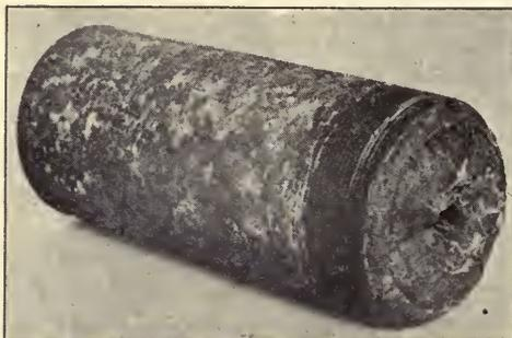
5-Inch Pipe Almost Closed by Scale
