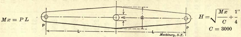
Allowance made for Hole h under 1 1-4 in. diameter. Stress in outer Fiber varies from 20,000 to 23,000 lbs. per sq. in.
