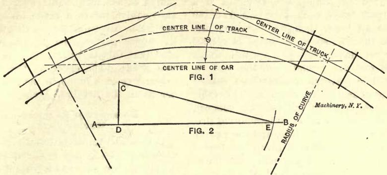
Put  $\sin \phi = \frac{\frac{1}{2} L}{R}$ , in which  $L$  = length center to center of bolsters and  $R$  = radius of curve, in feet, and the angle  $\phi$  can be laid out without using protractor. Erect to scale a perpendicular  $CD = \frac{1}{2} L$  on base line  $AB$ , Fig. 2. Then with  $C$  as a center, and radius  $R$  = radius of curve, to same scale, strike an arc intersecting  $AB$  at  $E$ . Angle  $CED$  is the angle required.
