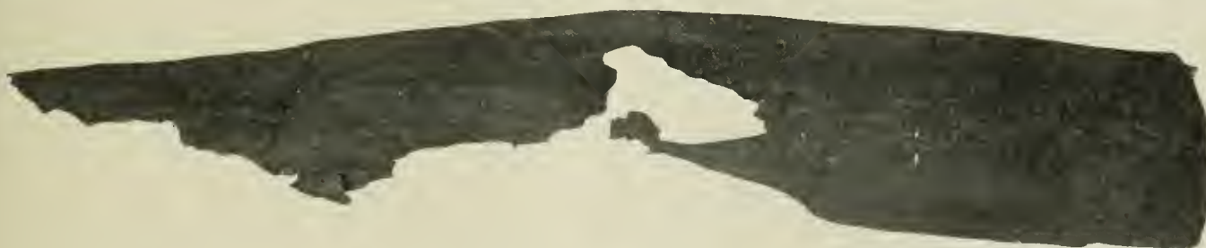
Service Gas Pipe Removed After Three Months.
