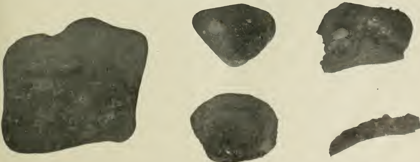
Pebbles Removed from Under Washington Street Showing Deposits from Cast-Iron and Lead Pipes.
