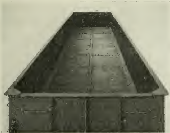
Arranged as Flat Bottom Gondola with Doors Up.
