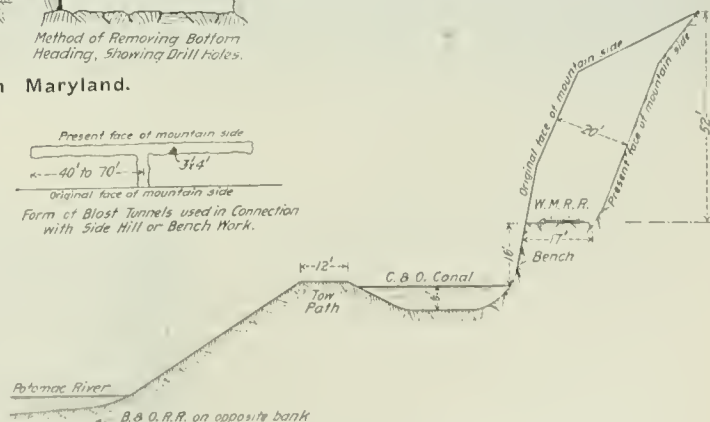
Typical Cross Section of Side Hill or Bench Work near Sideling Hill—Western Maryland.
