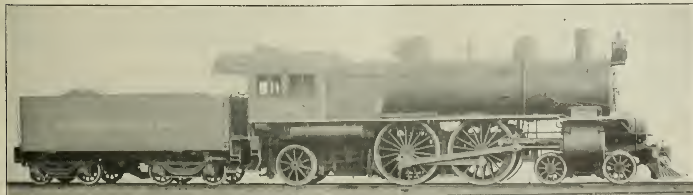
Four-Cylinder Balanced Compound Atlantic (4-4-2) Type Locomotive. Built by The American Locomotive Co.
