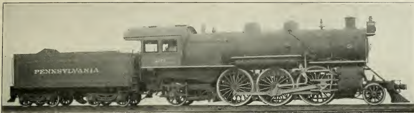
Prairie (2-6-2) Type Simple Locomotive. Built by The American Locomotive Co.
