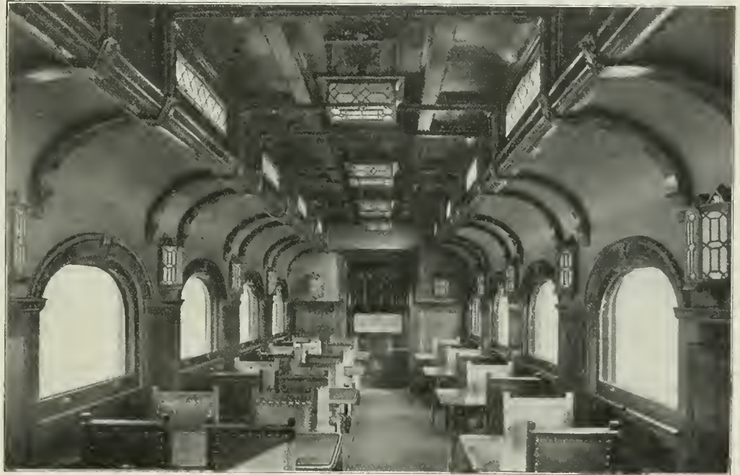
Interior of Dining Car Lighted With Inverted Mantle Pintsch Gas Lamps.
