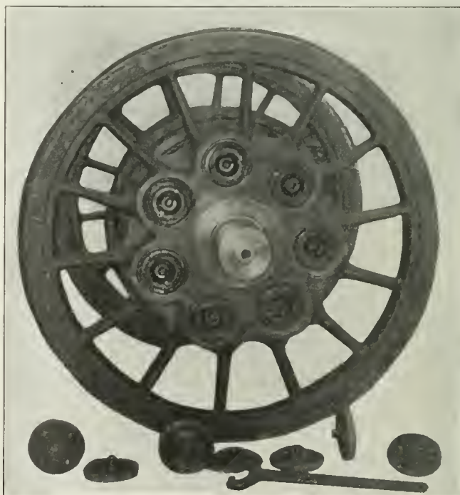
Driving Wheel With Caps Removed to Show Pockets for Driving Pins on Quill.
