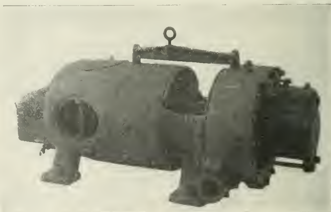
15 K.W. Turbine Generator Without Casing for Mounting in Baggage Car.
