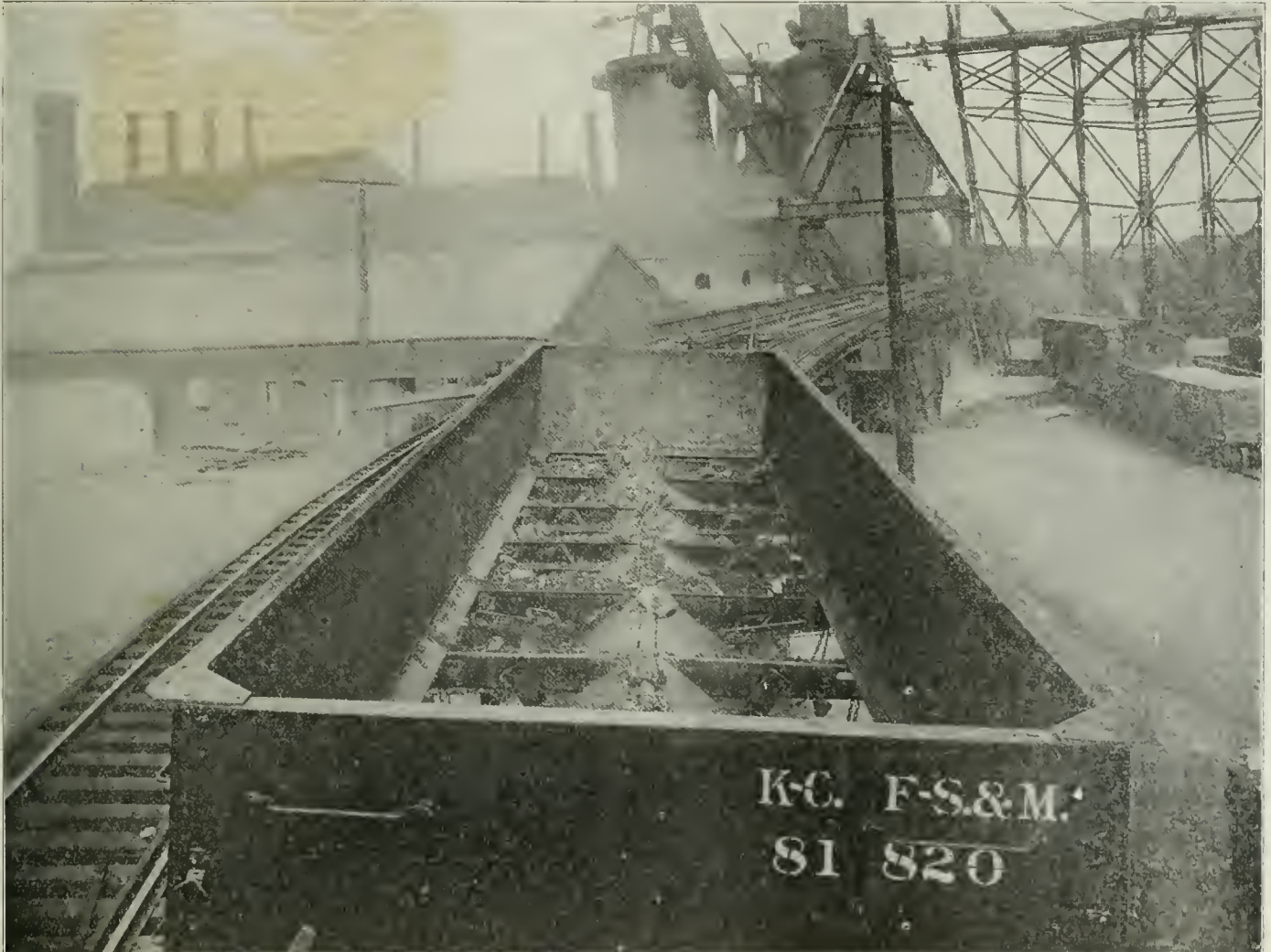
General Service Drop Bottom Gondola Car After Load Was Discharged by Gravity, No Shoveling.
