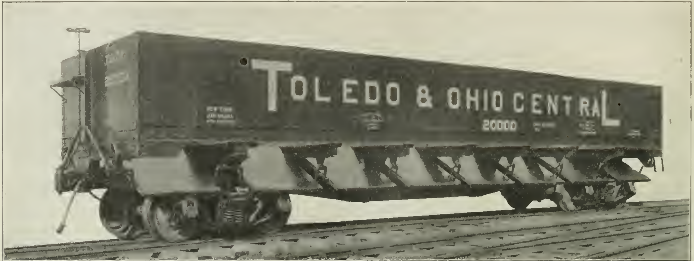
Ralston Flush-Floor Drop-Bottom Gondola Car for the Toledo & Ohio Central.
