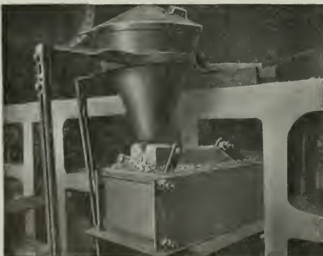
Mould and Crucible Ready for Pouring.
