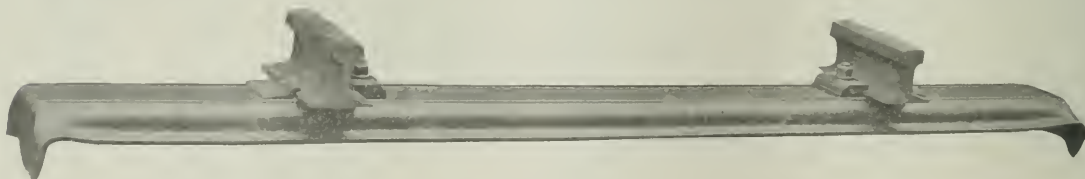
Fig. 1—Haarmann Steel Tie With Hook Plate Rail Fastening.
