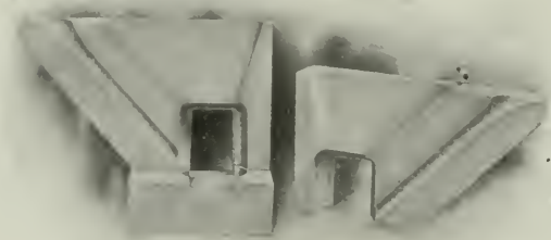
Parts of Firebrick Mould for Welding Locomotive Frames.
