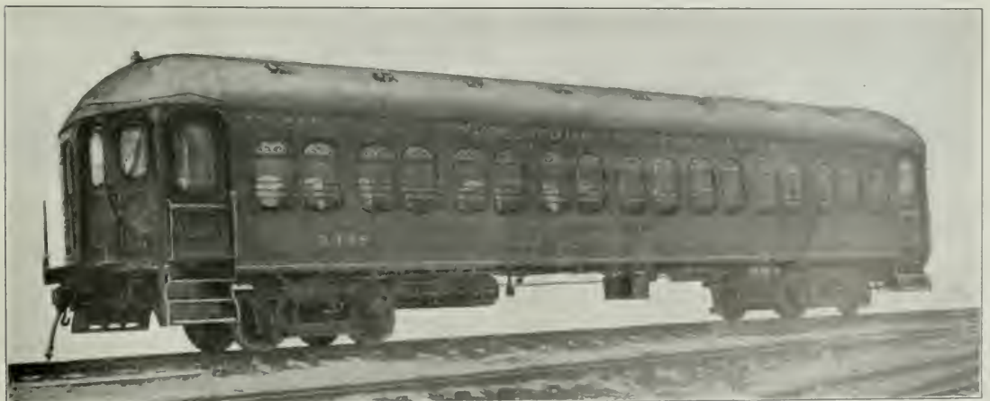
Wagenhals's Proposed Modification of Steel Passenger Car with Pressed Steel Side Plates and Curved Roof.
