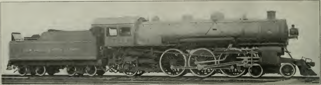
Pacific Locomotive with Combustion Chamber; Lake Shore & Michigan Southern.
