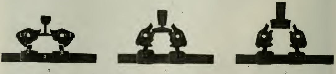
Fig. 3—Weaver's Rail Lock for Lift-Rails of Drawbridges.
