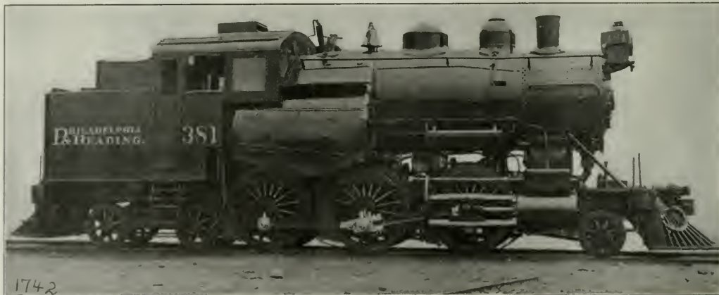
Type of Suburban Tank Locomotive Now in Use on the Philadelphia & Reading.
