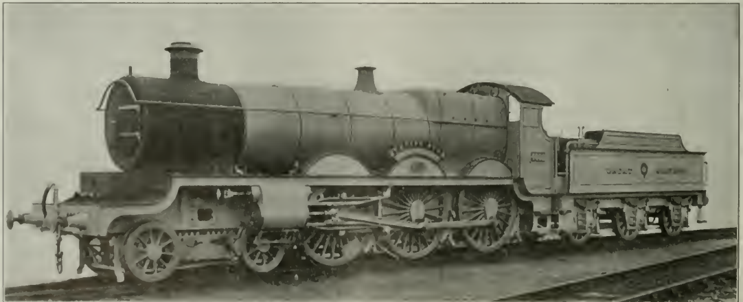
Four Cylinder Single Expansion Locomotive; Great Western Railway of England.
