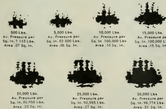
Contacts Between 36-inch Steel Tired Wheel and 80-lb. Rail.
