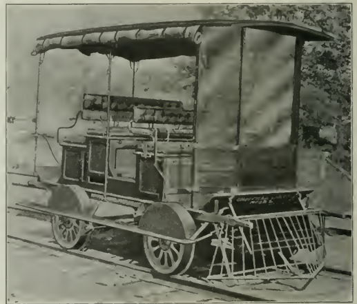
Gasolene Inspection Car; Fairbanks, Morse & Co.
