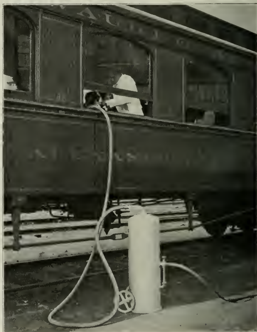
Cleaning Parlor Car by "Aero" Vacuum Machine.
