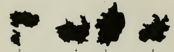
Contacts of 35-inch Steel Tired Wheel Under Cafe Car. Weight on Wheel, 6,075 lbs.
