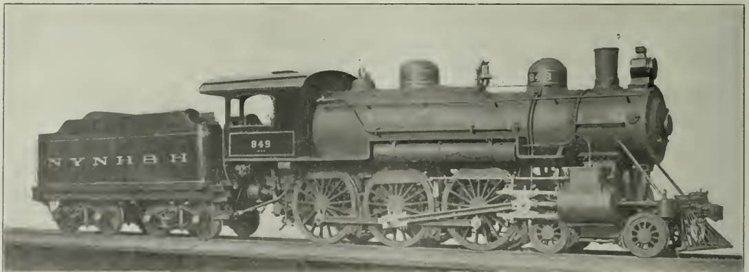
Ten-Wheel Passenger Locomotive for the New York, New Haven & Hartford; Built by the Baldwin Locomotive Works.
