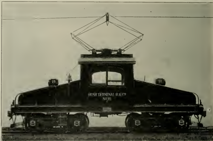
Electric Switching Locomotive; Bush Terminal Railroad.
