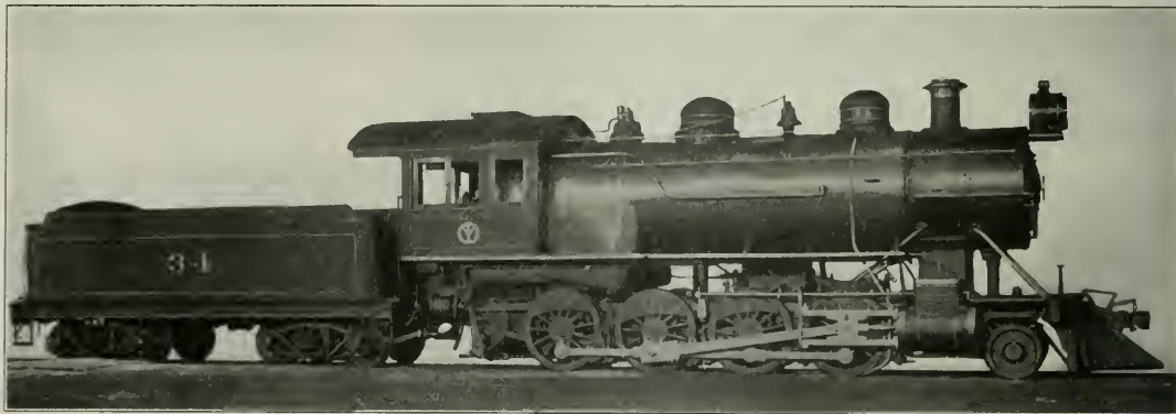
Consolidation Locomotive for the South Manchurian Railroads, Built at the Baldwin Works.
