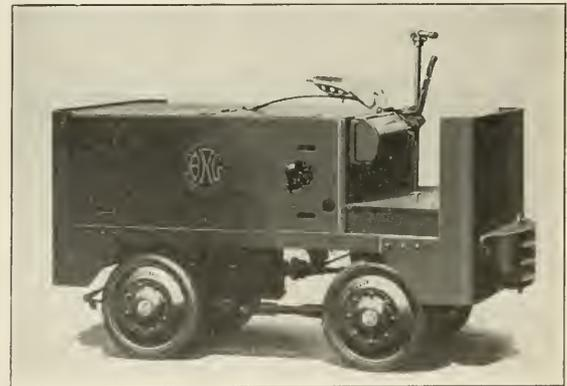
A Tractor of the Four-Wheel Drive, Four-Wheel Steer Type
