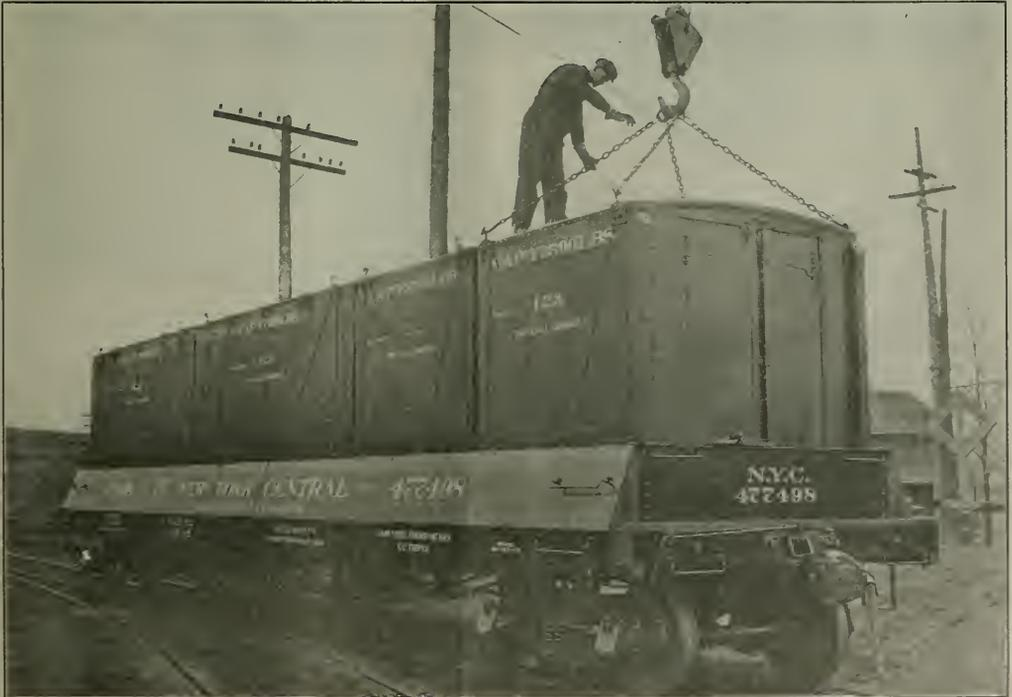
Car Loaded with Two Small and Two Large Freight Containers
