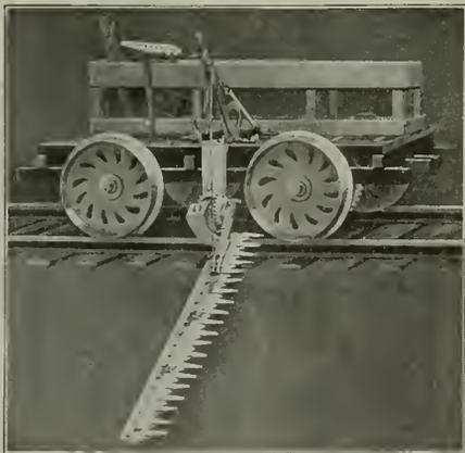
Motor Car With Mower Attached
