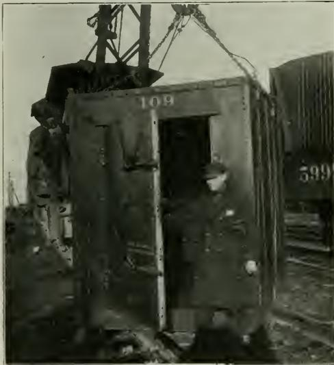
Empty Container Showing Interior and Door Construction
