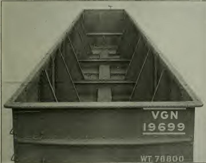
Interior of the Car Body, Showing Gusset Side Stakes, Bolsters and Cross Bearers
