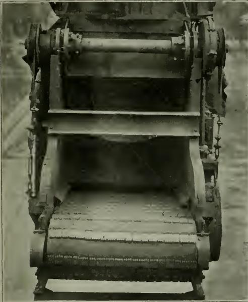
The Delivery End of the Trimmer, Showing the High Speed Belt
