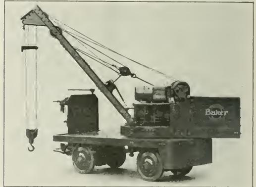
Three-Movement Electric Crane Truck
