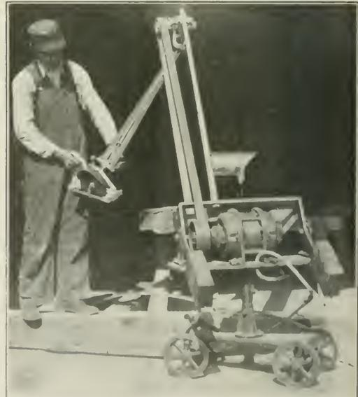
Flexway Machine Equipped for Ripping with Rip Gage
