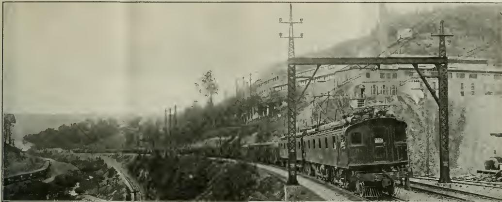
A 3,250-Ton Train on the Norfolk & Western Hauled by Two 11,000-Volt Alternating Current Locomotives
