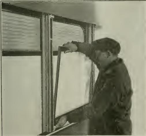
Window Sash May Be Removed from the Renitent Post Casings without the Use of Tools
