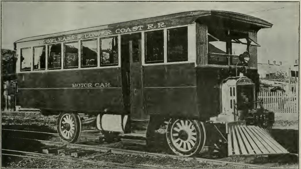
Four-Wheel Drive Rail Car Used on a Sixty-Mile Run Between New Orleans and Buras
