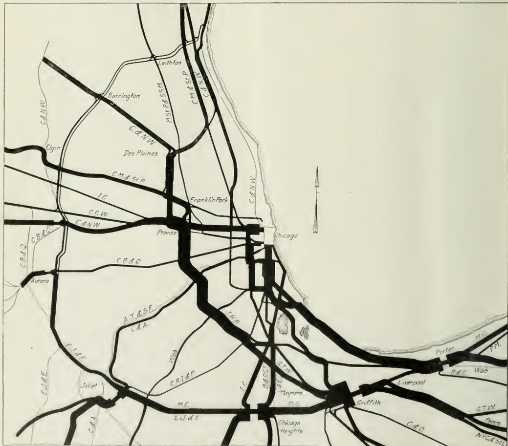
How Freight Traffic Could Be Routed—Plan for Proposed Rearrangement of Both Local and Through Operation—Showing Traffic Densities
