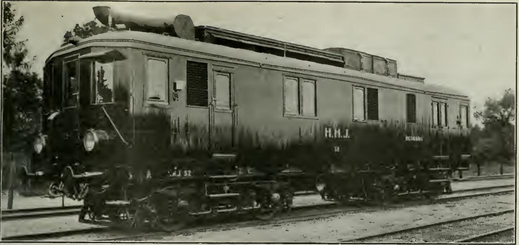
Swedish Diesel-Electric Motor Car of 250 Horsepower
