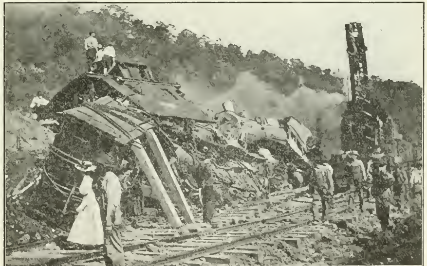
RESULT OF A "PITCH-IN," OR REAR COLLISION.
