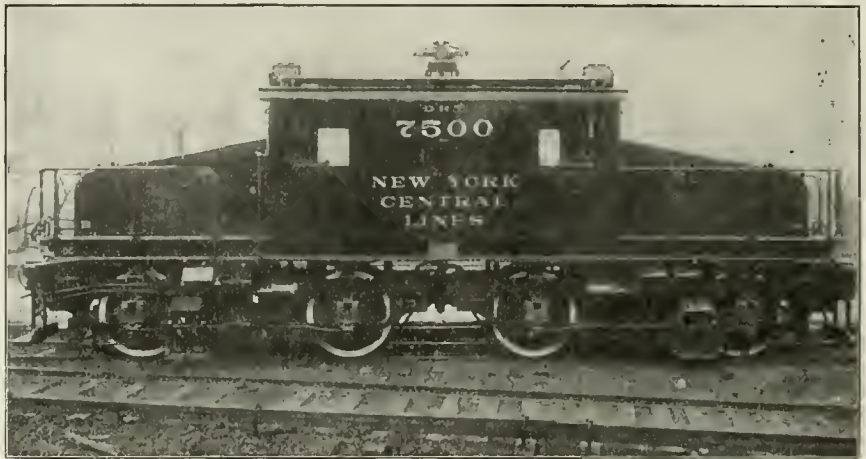
SIDE VIEW OF GENERAL ELECTRIC LOCOMOTIVE FOR DETROIT RIVER TUNNEL.
