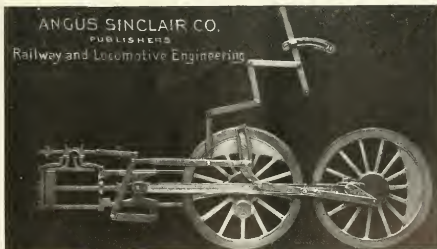
FIG. 1. FORWARD GEAR, LINK-BLOCK AT BOTTOM OF LINK.
