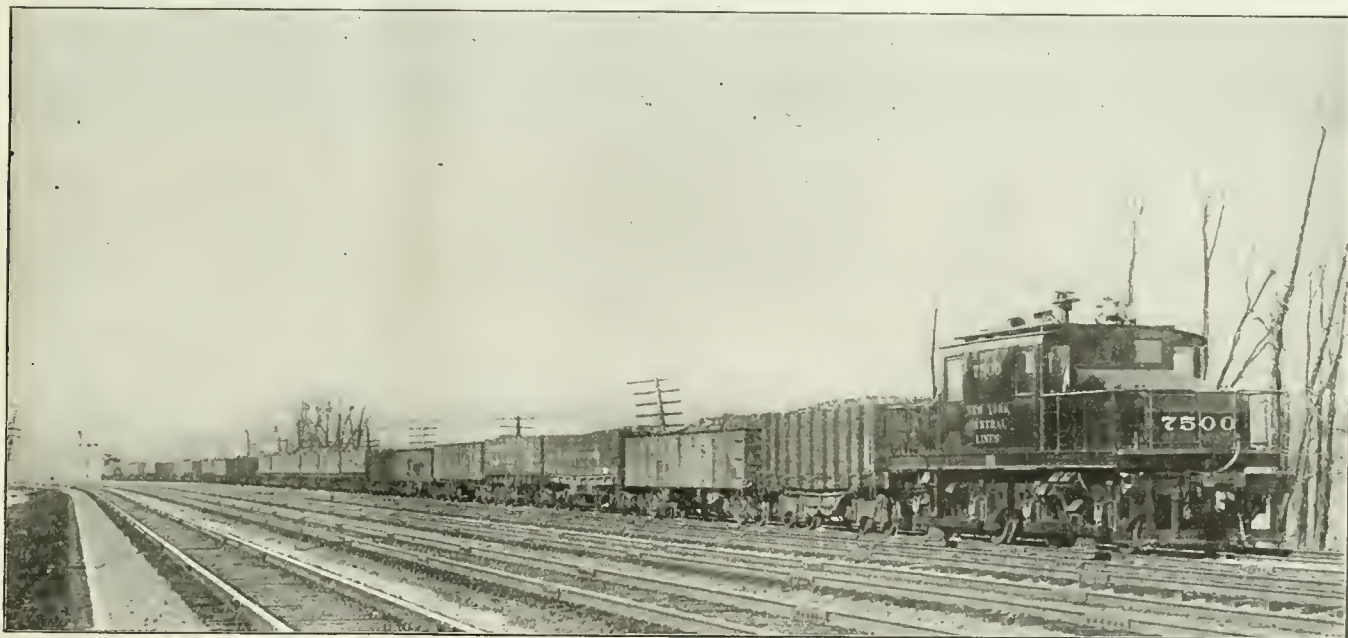
DETROIT RIVER TUNNEL ELECTRIC LOCOMOTIVE HANDLING 1,400-TON FREIGHT TRAIN.
