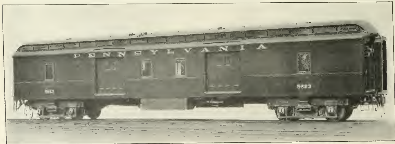
ALL-STEEL BAGGAGE CAR BUILT BY THE PRESSED STEEL CAR CO. FOR THE PENNSYLVANIA.
