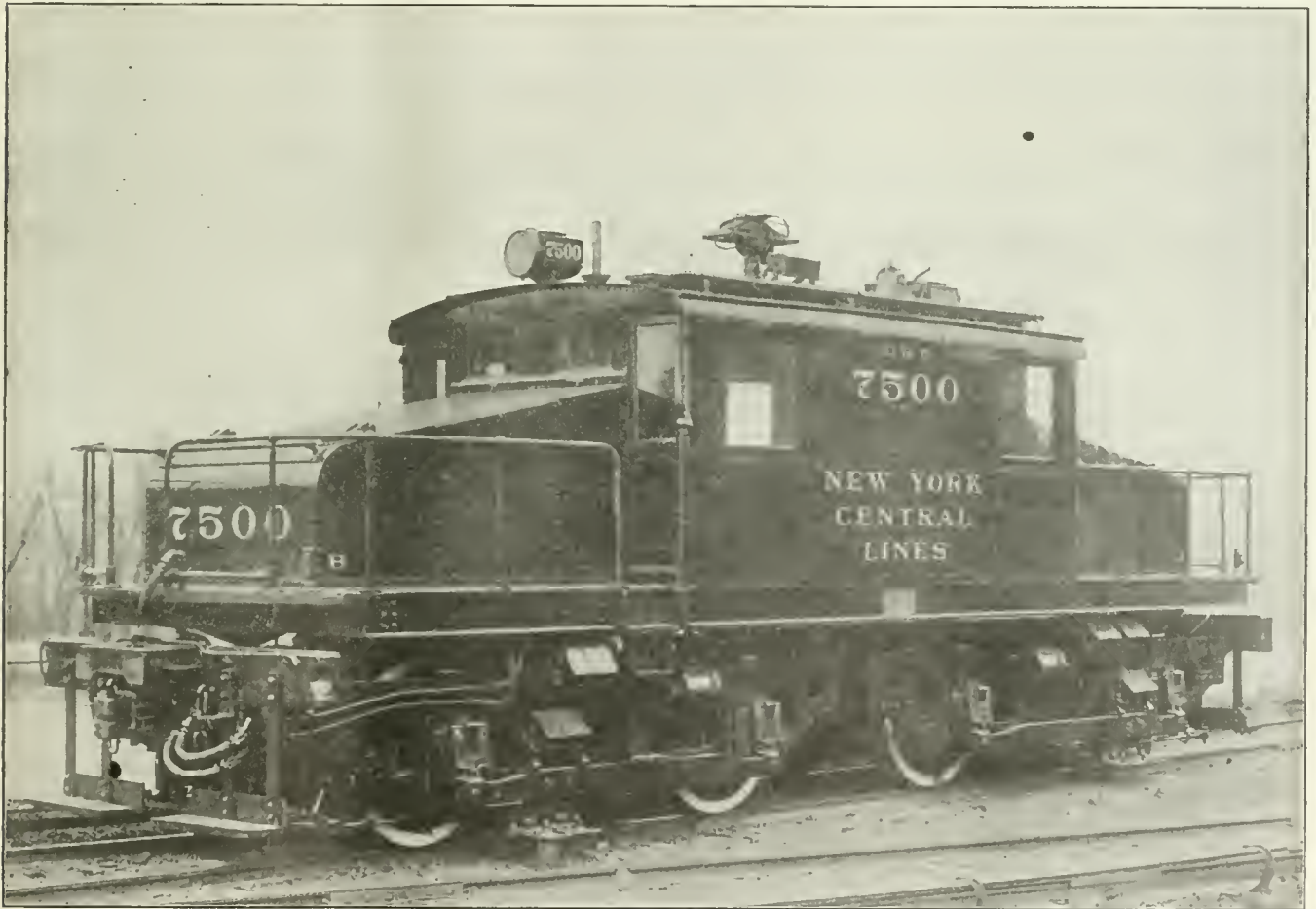
ELECTRIC LOCOMOTIVE FOR PASSENGER AND FREIGHT SERVICE IN THE DETROIT RIVER TUNNEL.
