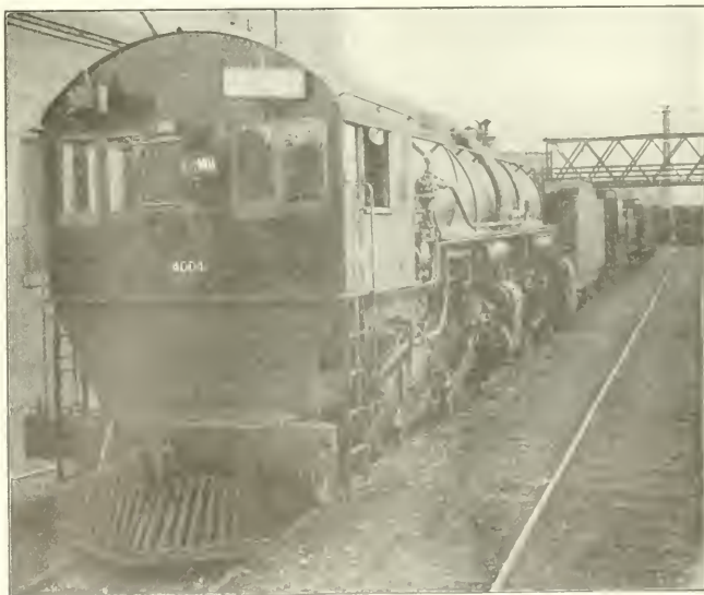
VIEW OF BALDWIN MALLET COMPOUND FOR THE SOUTHERN PACIFIC CO. THIS ENGINE RUNS CAB FIRST.
