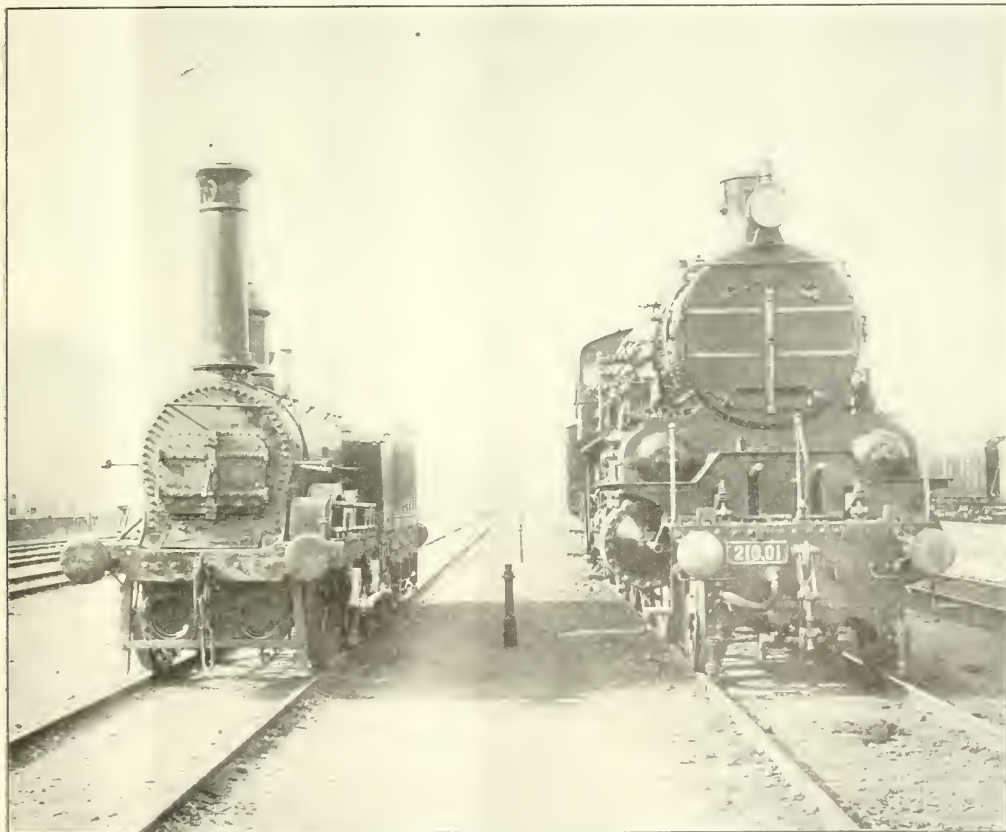
OLD ENGLISH ENGINE AND 4-CYLINDER GOLSZDORF COMPOUND FOR THE AUSTRIAN STATE RAILWAYS.
