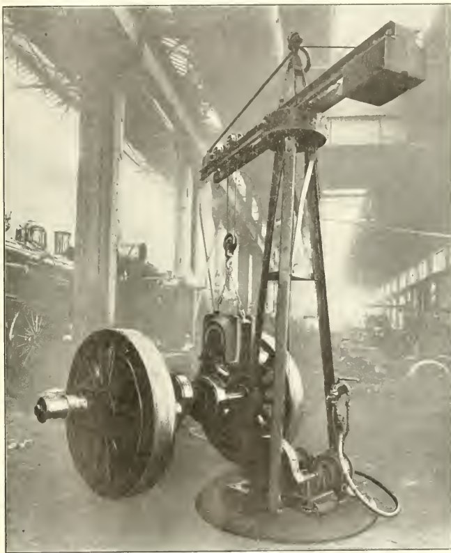
PORTABLE SHOP CRANE USED AT THE TRENTON SHOPS OF THE P. R. R.
