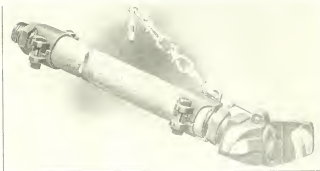
THE HEAVY-DUTY STEAM COUPLING, WITH LOCK.
