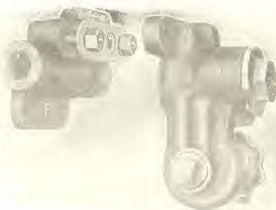
FIG. 1. DISTRIBUTING VALVE, ON RESERVOIR.
