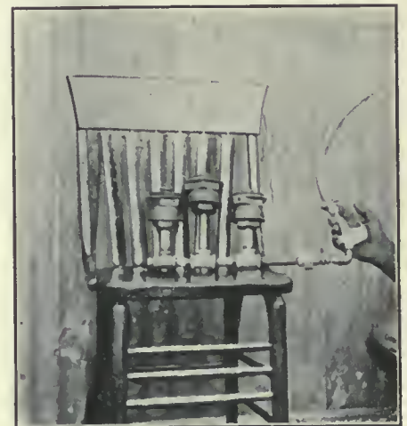
TESTING AND GRINDING RACK FOR PISTON PACKING RINGS.
