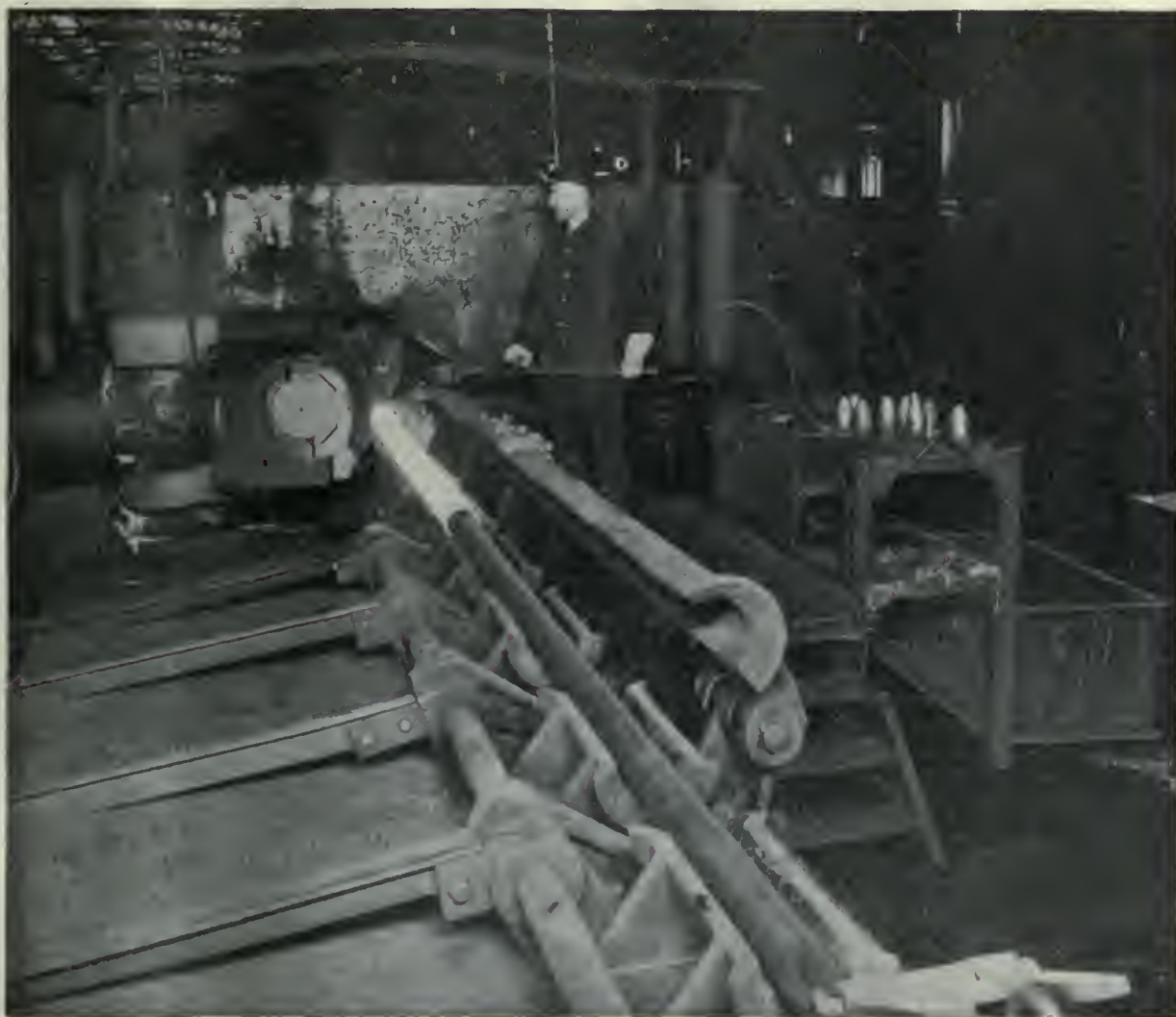
ROUGH TUBE COMING THROUGH PIERCING MILL
