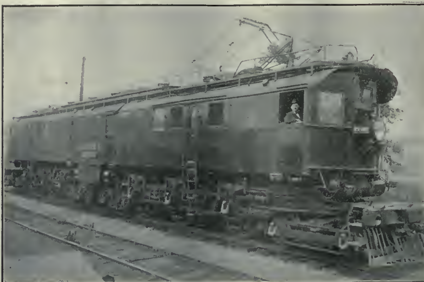
275-TON PASSENGER LOCOMOTIVE—CHICAGO, MILWAUKEE & ST. PAUL RAILROAD.
