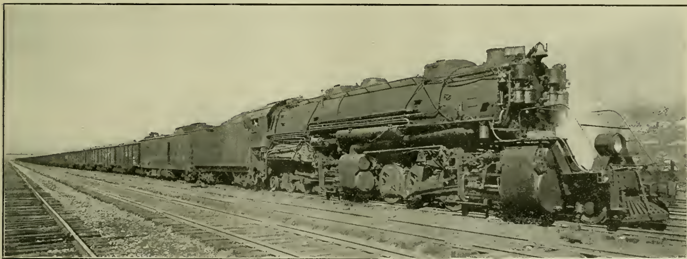
TEST TRAIN OF SEVENTY 100-TON CARS EQUIPPED WITH AUTOMATIC STRAIGHT AIR BRAKE, WITH TOTAL WEIGHT OF 9,355 TONS, NORFOLK & WESTERN RAILWAY
