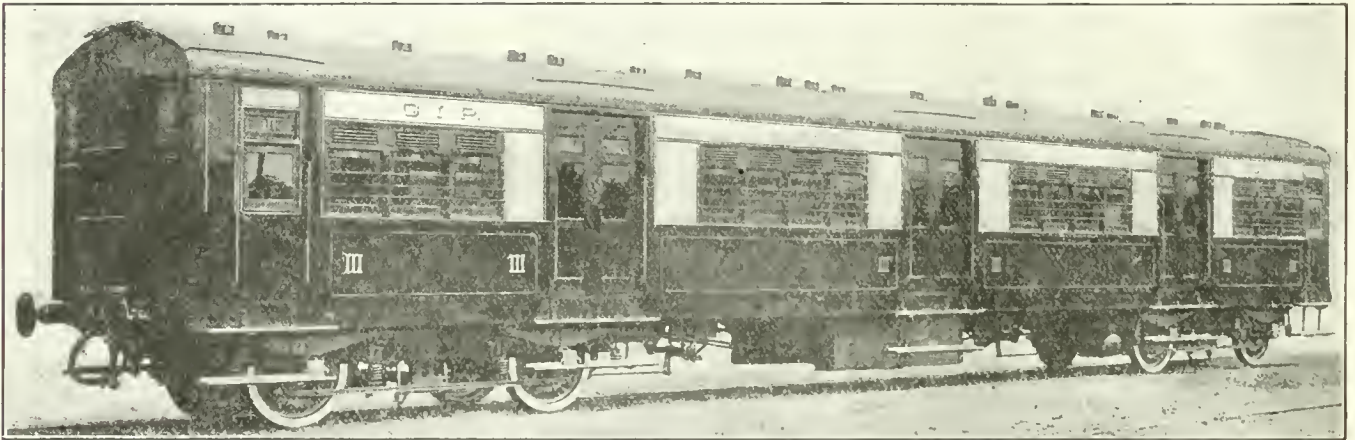
NEW STEEL CAR FOR SUBURBAN SERVICE ON THE GREAT INDIA PENINSULA RAILWAY
