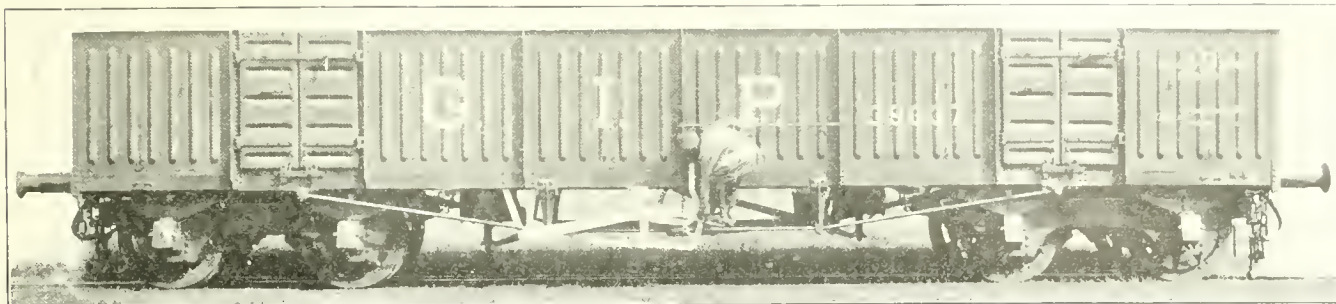
OPEN 40-TON WAGON, SHOWING THE HAND BRAKE BEING OPERATED BY NATIVE SHUNTER
