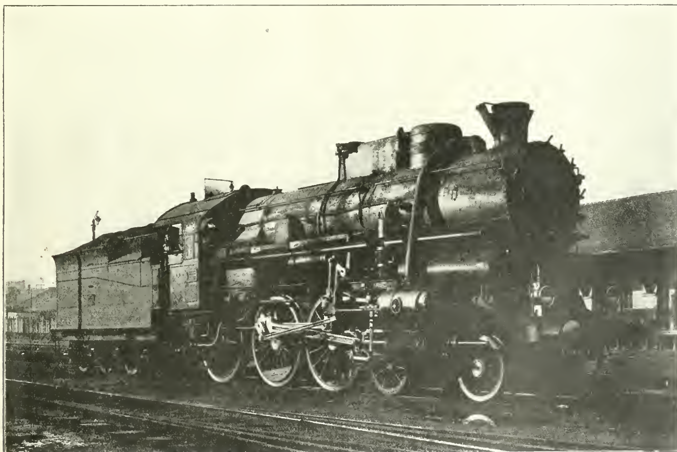
ROYAL HUNGARIAN STATE RAILWAYS 4-6-0 TYPE EXPRESS LOCOMOTIVE EQUIPPED WITH BROTRAN BOILER, WATER TUBE FIREBOX, LOOP WATER PURIFIER AND PREHEATER
