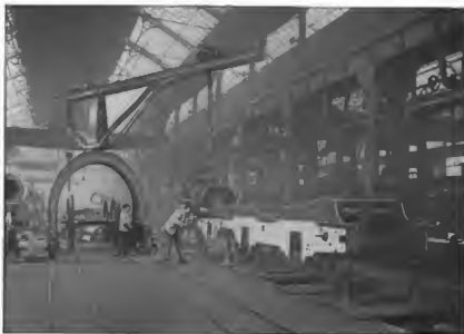
FIG. 24. HYDRAULIC RIVETER FOR FRAMES.
