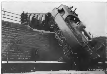
WHAT HAPPENED IN VIENNA, AUSTRIA, THROUGH OPEN SWITCH AND DEFECTIVE BRAKE.
