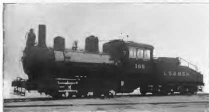
Cylinders, 19 x 26; Weight on Drivers, 122,700 lbs.; Total Weight, 122,700 lbs.
