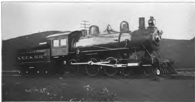
VANDERBILT ENGINE WITH CORRUGATED FURNACE.
