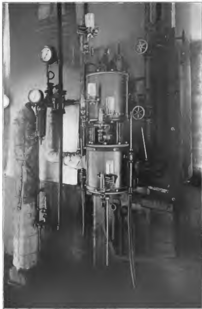
9 1/2-INCH AIR PUMP AT CORNELL UNIVERSITY RIGGED UP TO TEST EFFICIENCY OF A WATER JACKET ON THE AIR CYLINDER.
