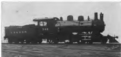
Cylinders, 19½ x 30; Weight on Drivers, 120,000 lbs.; Total Weight, 154,000 lbs.
