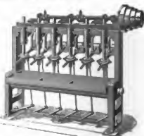
Acme 1/2 inch Six Spindle Nut Tapper. Net Weight, 3,800 lbs.
