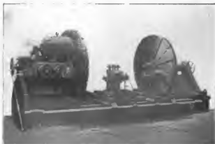
Double Locomotive Driving Wheel Lathe—Electrically Driven.
