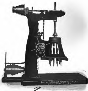
Eight Spindle Multiple Drill for 1 1/2 inch Drills. No. 25.
