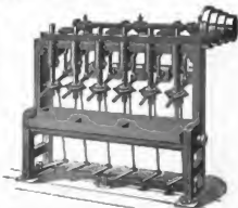
Acme 1 1/2 inch Six Spindle Nut Tapper. Net Weight, 3,800 lbs.
