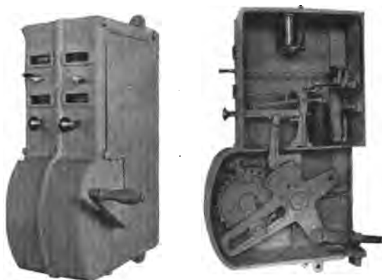
Three-quarter and sectional view of the controlled manual signal mechanism made by the General Railway Signal Company. The signal is cleared by manipulation of the handle shown in the first picture, under the proper circumstances.
