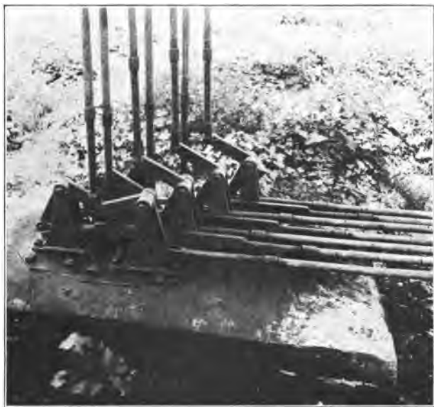
Showing method of transmitting motion from pipe-run on the ground to signals on a bridge.
