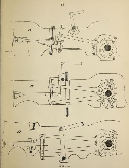
links then extend up to them; thirdly with no saddles, the weigh-shaft above, and the swing-links reaching down to the bottom of the link and coupling on to the same pin as the back-gear eccentric rods; and, fourthly, the weigh-shaft, etc., below, with the swinglinks coupled to the tore-gearing eccentric rod pin at the top of the link. The first two methods are most common, the other two, however, are often met with.
