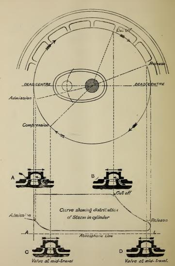
pressure when the point of release is reached; here the valve opens to exhaust, and the cylinder is emptied by the return stroke of the piston. The "back pressure" or resistance to movement of the piston is shown by the base line of the diagram immediately above the atmospheric line drawn to illustrate the condition of affairs which would exist if the cylinder had its end open to the atmosphere. C and D show the position of the valve at midtravel.
