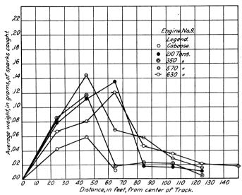
Fig. 2.—Average weight of sparks from the Switching locomotive
