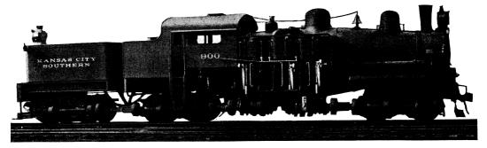
Fig. 1. 190-Ton Geared Locomotive for Switching Service on 7% Grades and  $60^{\circ}$  Curves; Kansas City Southern Ry.
