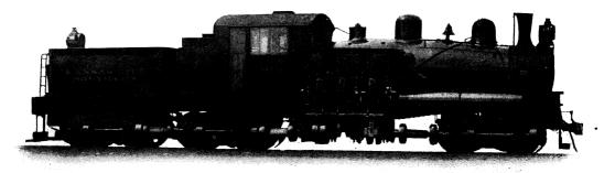
FIG. 2. 140-TON GEARED LOCOMOTIVE FOR SWITCHING ON 7% GRADES AND 60° CURVES; KANSAS CITY SOUTHERN RY.
