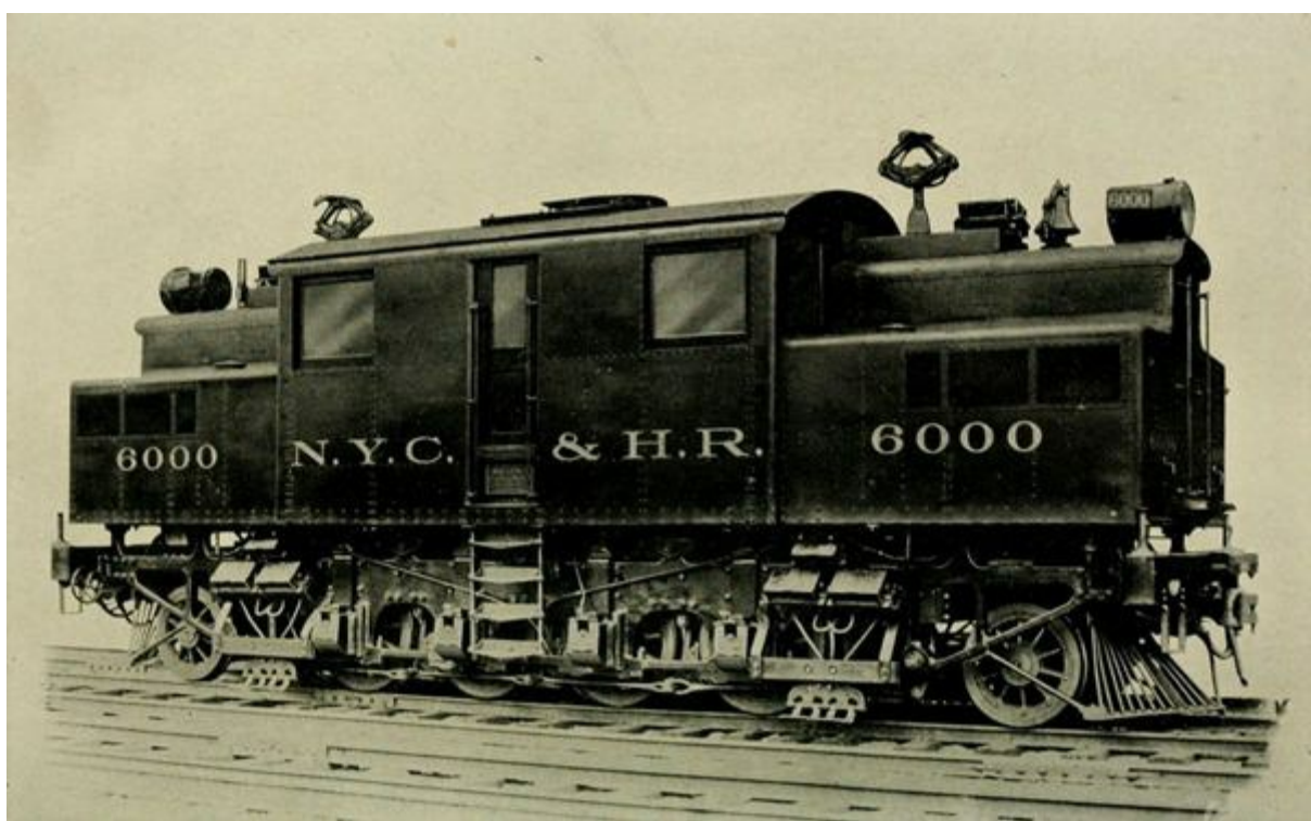
HIGH-SPEED, DIRECT-CURRENT PASSENGER LOCOMOTIVE BUILT BY THE GENERAL ELECTRIC COMPANY FOR TERMINAL SERVICE OF THE NEW YORK CENTRAL AT THE GRAND CENTRAL STATION
